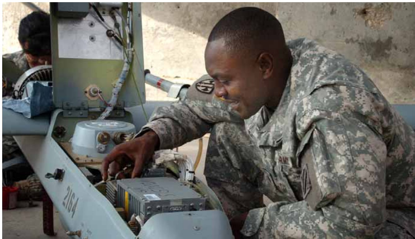
Sgt. Cliff Nji, with Co. A, 4-3 BSTB, conducts a preventive maintenance daily Dec. 21 after a Shadow 200 RQ-7B unmanned aerial vehicle landed. PMD is performed after every flight to check if the aircraft was damaged during its flight and to prepare it for its next mission.
