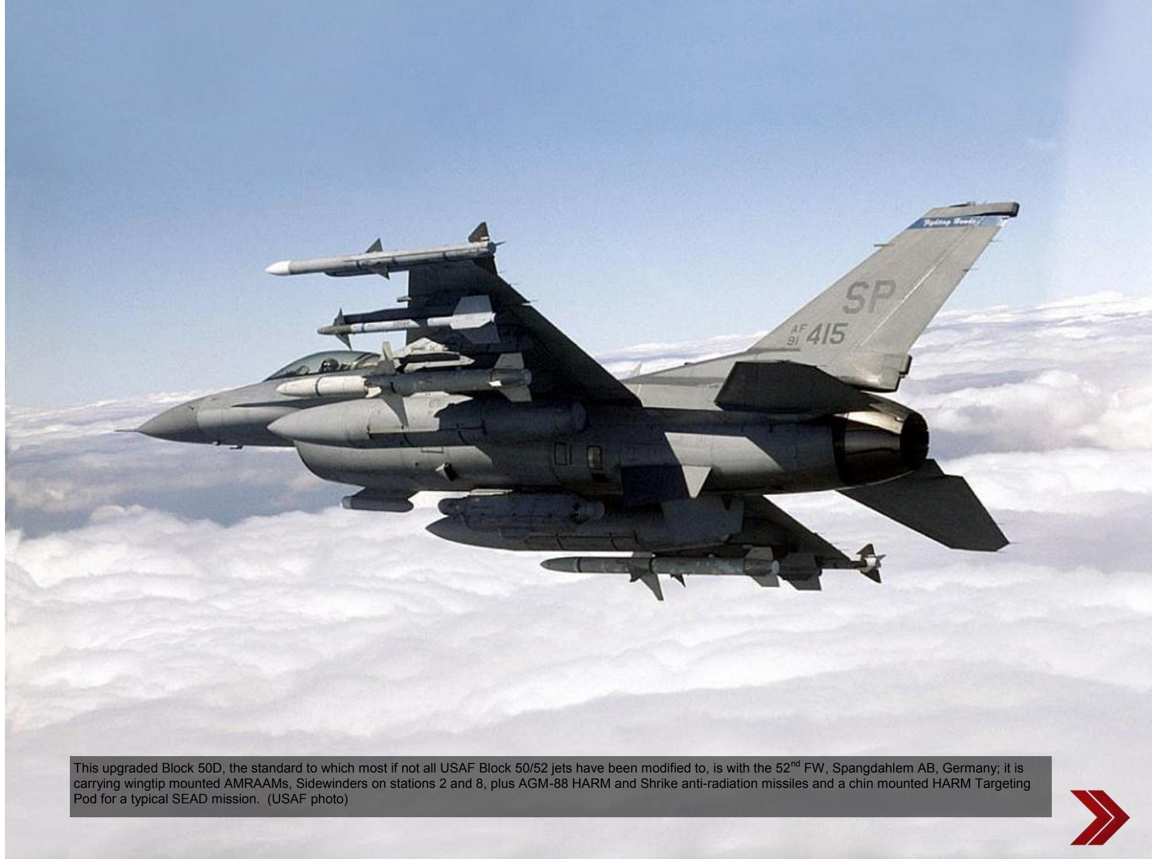
This upgraded Block 50D, the standard to which most if not all USAF Block 50/52 jets have been modified to, is with the 52<sup>nd</sup> FW, Spangdahlem AB, Germany; it is carrying wingtip mounted AMRAAMs, Sidewinders on stations 2 and 8, plus AGM-88 HARM and Shrike anti-radiation missiles and a chin mounted HARM Targeting Pod for a typical SEAD mission. (USAF photo)
