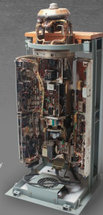
AIM-7E-2 Sparrow III Guidance System Number R11641-b-2 from the NSWC Corona Archive
