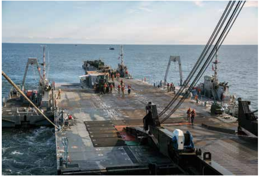
A roll-on/roll-off discharge facility and an Improved Navy Lighterage System are attached to USNS 1ST LT Jack Lummus (T-AK 3011) with ropes and a ramp during a Maritime Prepositioning Force Exercise allowing Marines with Combat Logistics Regiment 25 and Sailors with Naval Beach Group 2 to offload the Lummus using in-stream methods off the coast of Marine Corps Support Facility Blount Island, Florida. (U.S. Marine Corps photo by Sgt. Shawn Valosin/Released)
