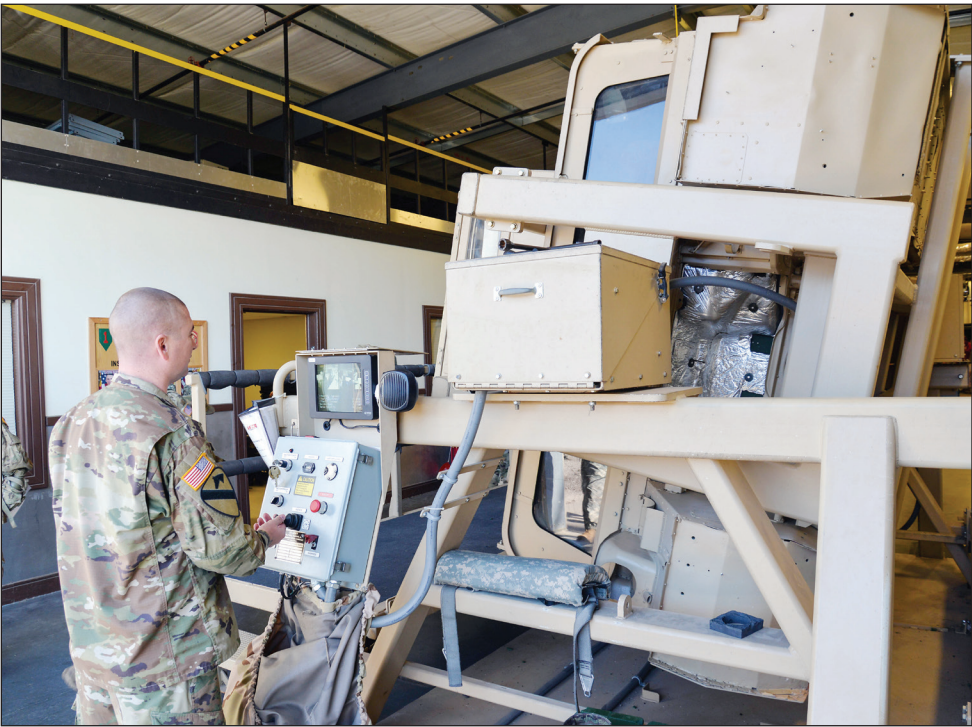
Staff Sgt. Luke Sulak, a Humvee Egress Assistance Trainer operator, rotates the HEAT with Soldiers inside April 6 at Fort Riley. Sulak rotated the vehicle several complete turns to simulate rolling down a hill or into a ditch before coming to rest.
