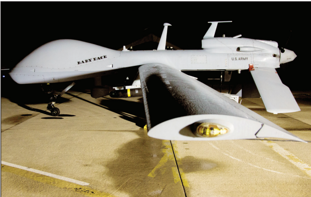
An MQ-1C Gray Eagle, a long-endurance platform able to fly for nearly 27 hours at speeds of up to 150 knots while carrying up to four AGM-114 Hellfire missiles, is shown April 1 in Al Asad, Iraq. U.S. Army Soldiers assigned to Company D, 10th Aviation Regiment, 10th Mountain Division, deployed to Al Asad, Iraq, in support of Combined Joint Task Force - Operation Inherent Resolve, provide fire support on the battlefield from the skies. CJTF-OIR is the global Coalition to defeat ISIS in Iraq and Syria.
