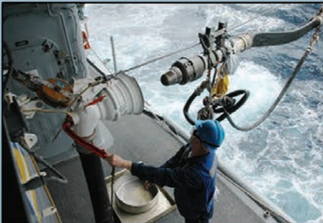
A deck rigger aboard USS COMSTOCK (LSD 45) ensures a proper lineup of a fuel probe and receiver during underway replenishment.
