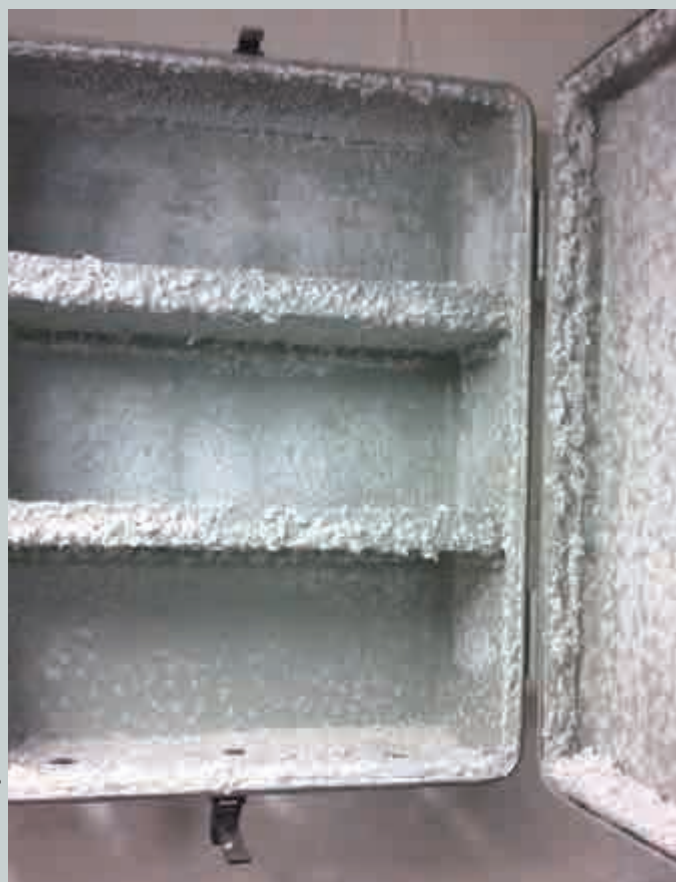
An example of an improperly maintained hypochlorite locker.
