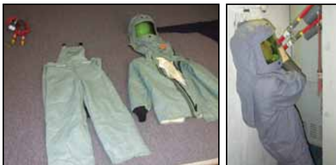
New, high-voltage PPE and faceshield (left) and full arc flash suit, including a high-voltage metering probe, for use with 4,160-volt system. Photos courtesy of the author.
