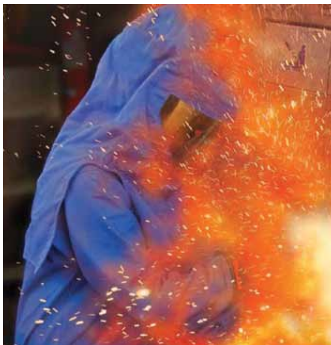
Arc flash personal protective equipment (PPE) is tested during arc flash of 5,000-volt circuit. Photo courtesy of ArcFlashPPE.com.
