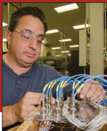
Anthony Tolerico, electronics technician, tests a SATCOM cable using the Drive In Theater Manufacturing Company (DITMCO) test set.
