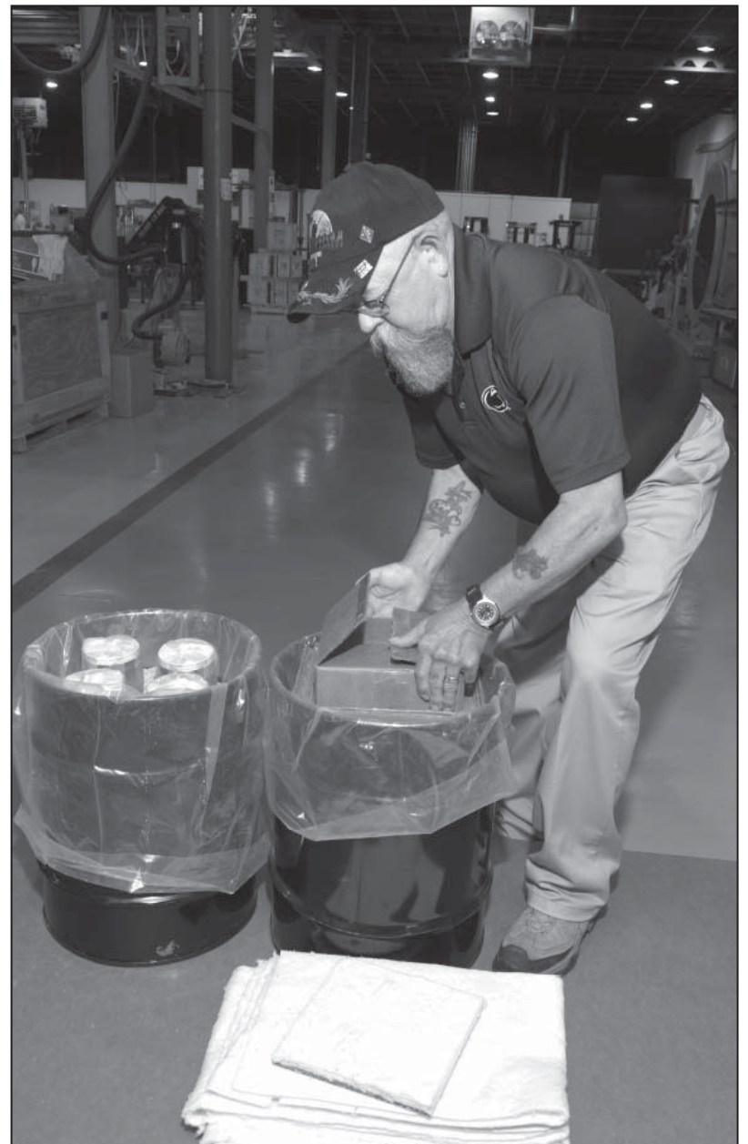
Jim Mott, systems engineer, demonstrates how new packaging methods can save money and protect the environment when shipping liquid hazardous materials.
