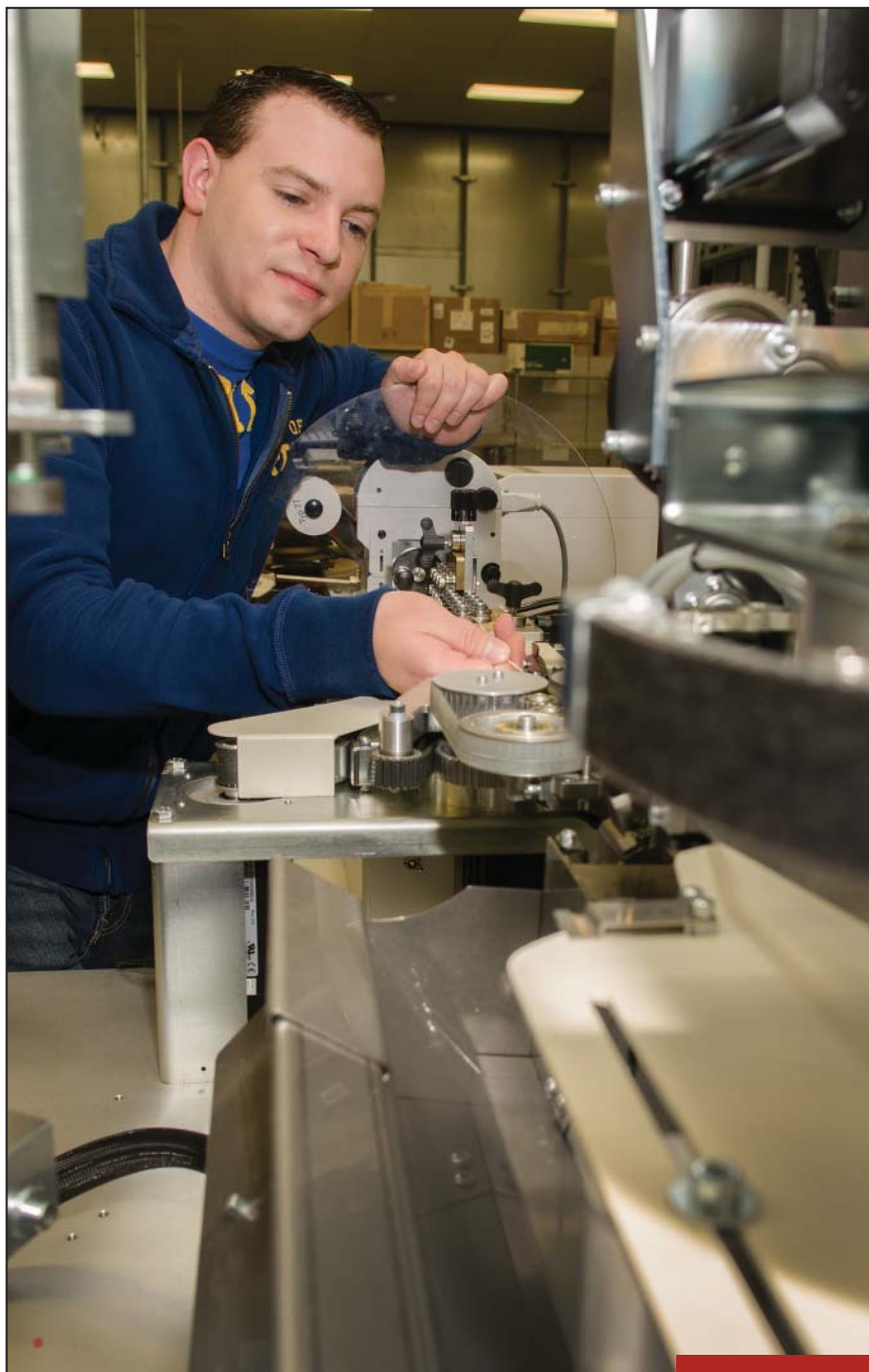
Matt Check, electronics technician, sets up the Schleuniger Crimp Center to mark and strip wires for the Common Remotely Operated Weapon Station (CROWS) identification box.
