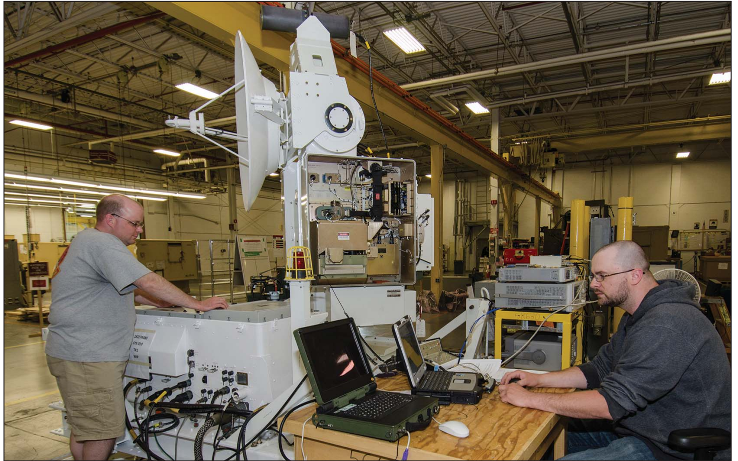
Left, electronics mechanics Anthony Dennis and Robert Slater conduct a system performance check on a Air Force Unmanned Threat Emitter (UMTE) training system after it was overhauled and reassembled. Site acceptance testing for the first overhaul was performed at a remote training range in the Alaska wilderness. (Photo by Steve Grzedzinski)
