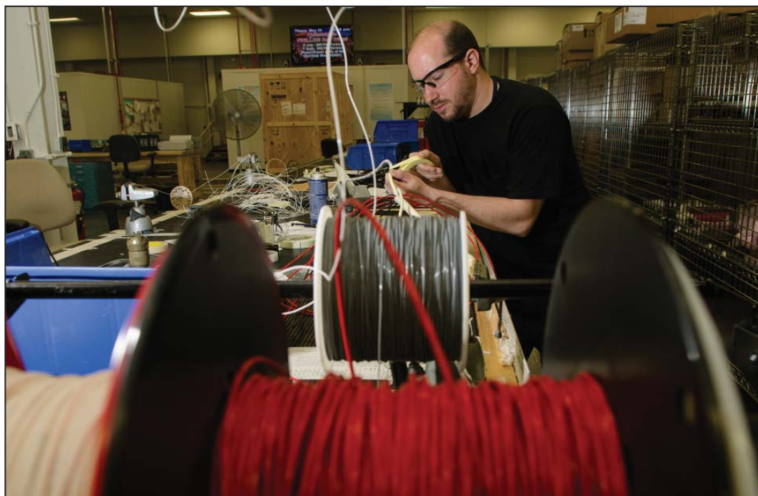
Scott Capman, electronics technician, bundles CROWS cables.
