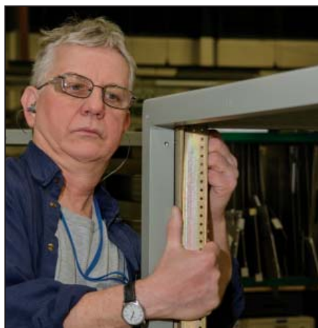
Sheet Metal Mechanic James Medwetz installs a pin bracket on a power supply rack for an AN/ASM-146 Electronics Shop Van.
