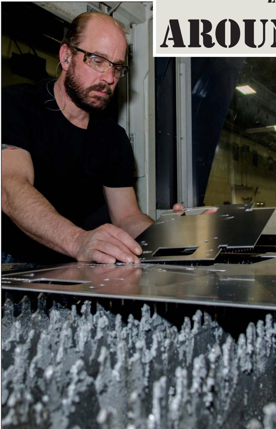
Mark Nizich, metal forming machine operator, uses a laser cutting machine to cut the base for a satellite communications antenna mount.
