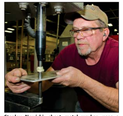
Stanley Nowicki, sheet metal worker, uses a press machine to install a clinch nut. The nuts are designed to be installed into a pre-drilled or punched hole so it is flush on the back side.
