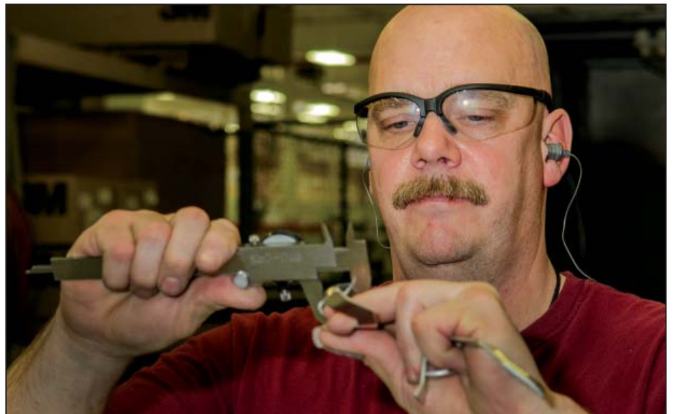
Frederick Teufert, sheet metal mechanic leader, uses a dial caliper to get a precise measurement on a bracket for the Personnel Armor System for Ground Troops helmet clip.
