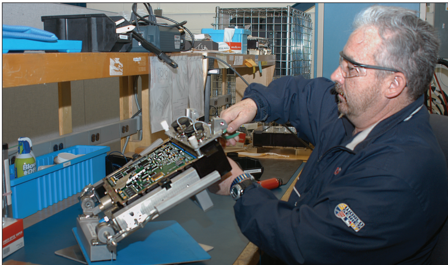
William Germek, work leader in the Command, Control and Computers/Avionics Directorate's Airborne Communications/Instrument Branch, disassembles a T-55 Electronic Control Unit to replace a circuit card assembly and prepare the unit for mechanical overhaul inspection. (Photo by Justin Eimers)
