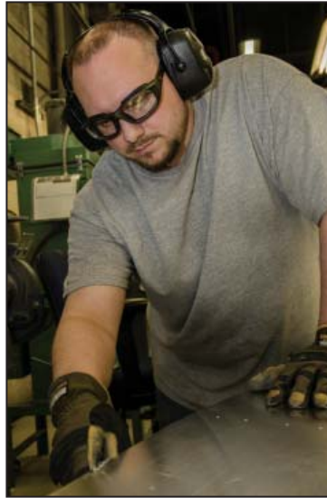
Robert Migatulski, metal forming machine operator, deburrs a fender weldment for an AN/TPQ-36 Firefinder.
