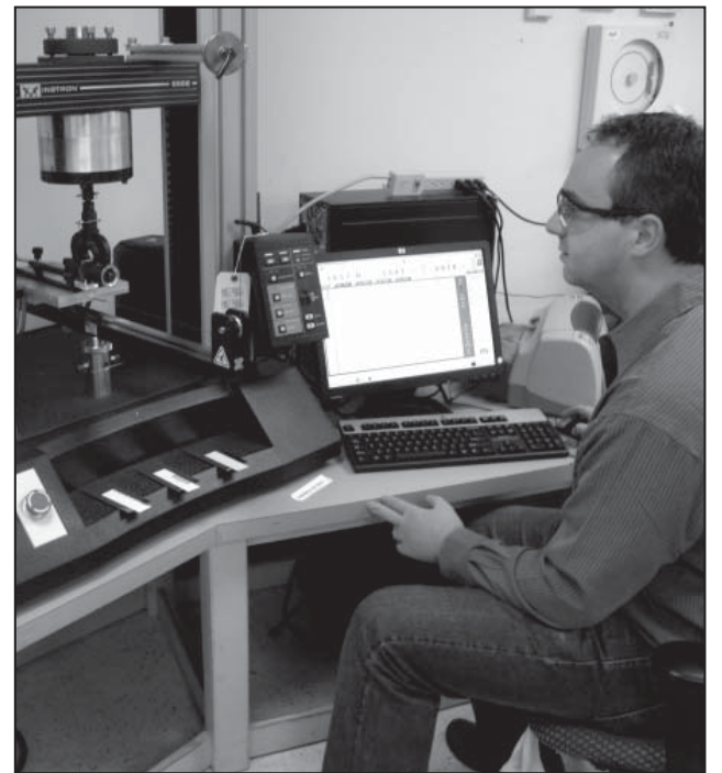
Andrew Gesford, general engineer, performs a 90-degree peel adhesion test on pressure-sensitive tape. (U.S. Army photo)
