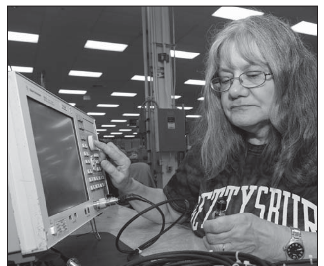
Wanda Walb-Gower, electronics worker, tests Nett Warrior RF extension cables on the network analyzer. Walb-Gower works in the Satellite Data Cable Branch. (Photo by Steve Grzezdzinski)
