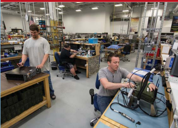
From left, Electronics Mechanics Gerard Daniels and Joe Gigliotti repair a transmitter and power supply, respectively, while Michael Lloyd performs an electrical test on a multiband radio.
