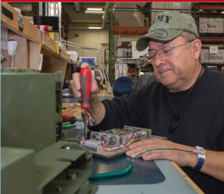
Arthur Caicedo, electronics mechanic, repairs an electrical mounting base.
