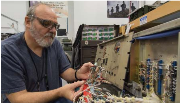
Ray Nardelli, electronics mechanic helper, tests the wiring harness on a Rockwell Collins Radio.
