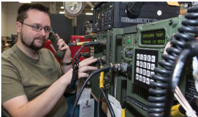
Electronics Worker James Solomon performs an electrical test on a radio used in the TRC-190 High Capacity Line of Sight Communications Terminal.
