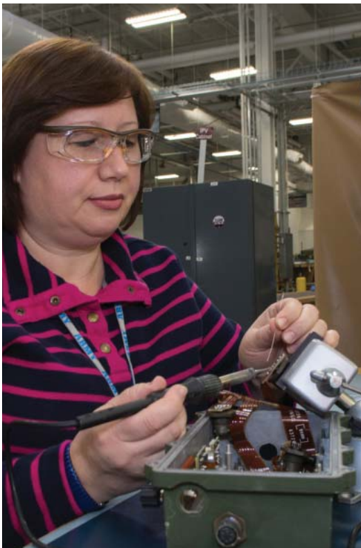
Electronics Mechanic Yelena Raykhel performs mechanical repairs on a master control station, a component of the vehicular intercom system.
