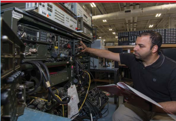
Electronics Mechanic Raul Genao tests an amplifier coupler on the AN/GRC-206 test rack.
