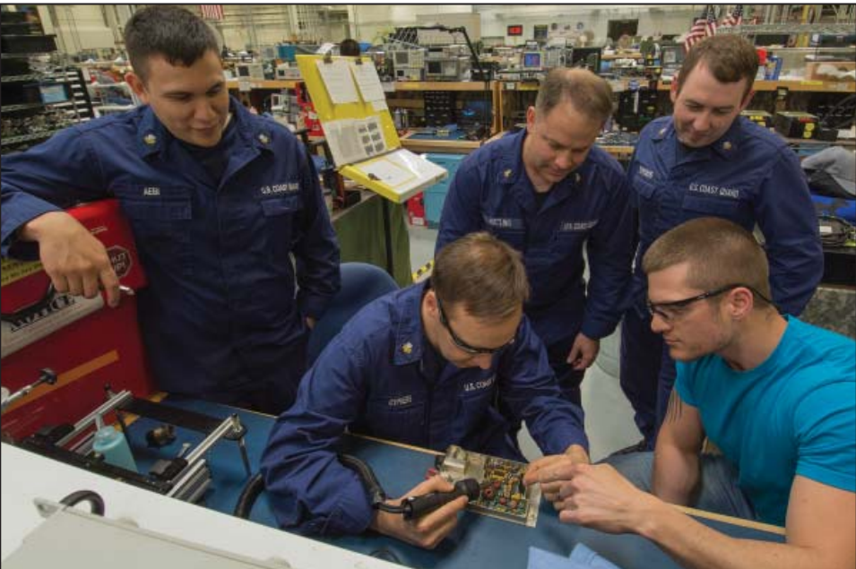
From left, Petty Officer 2nd Class Brian Aebi, Petty Officer 1st Class Phil Cyphers, Chief Petty Officer Daniel Nietling and Petty Officer 2nd Class Bjorn Tovsrud practice soldering on a Single Channel Ground and Airborne Radio System (SINCGARS) power supply with the instruction of Electronics Worker Joseph Rossi. Rossi works in the C4ISR Directorate’s SINCGARS Section. (Photo by Steve Grzezdinski)
