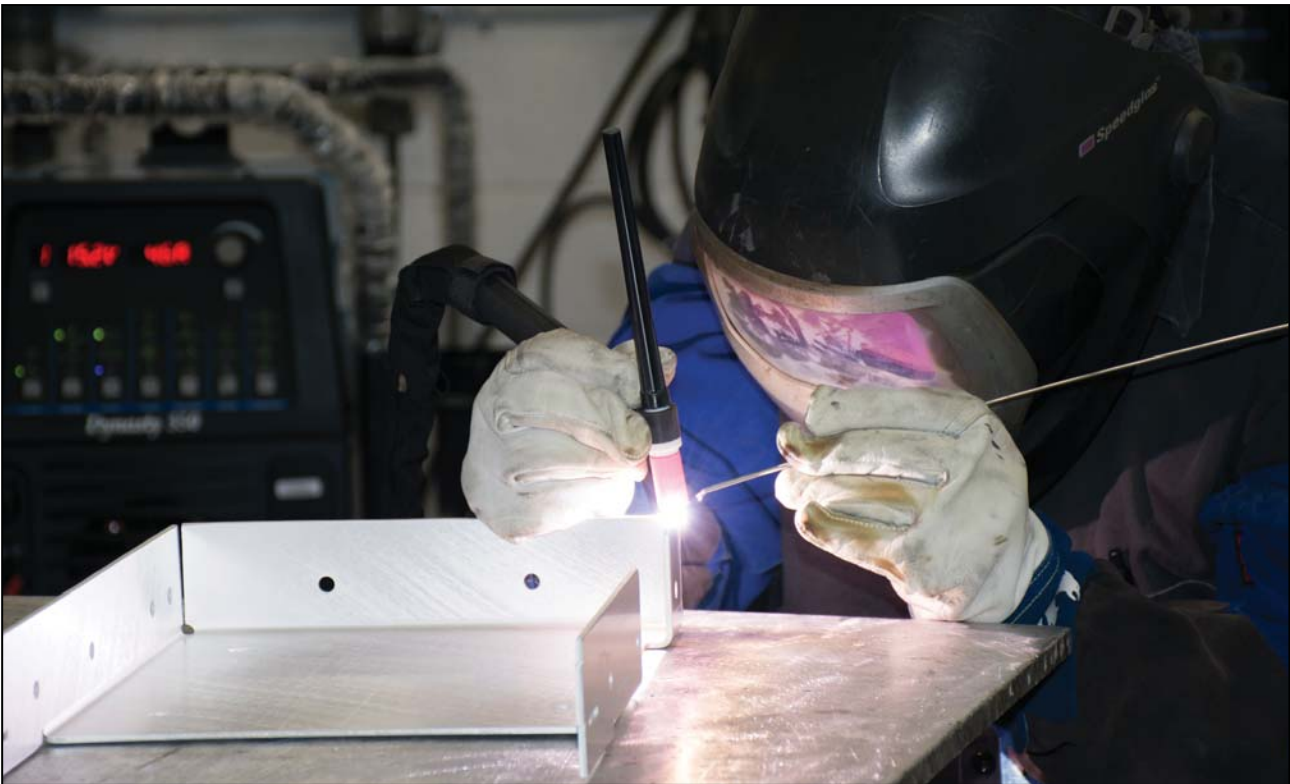
Welder Robert Knecht uses the depot’s new Miller Dynasty 350 tungsten arc welder on a Blue Force Tracking windshield mount assembly. The Systems Integration and Support Directorate plans to purchase four new Dynasty machines. (Photo by Justin Eimers)
