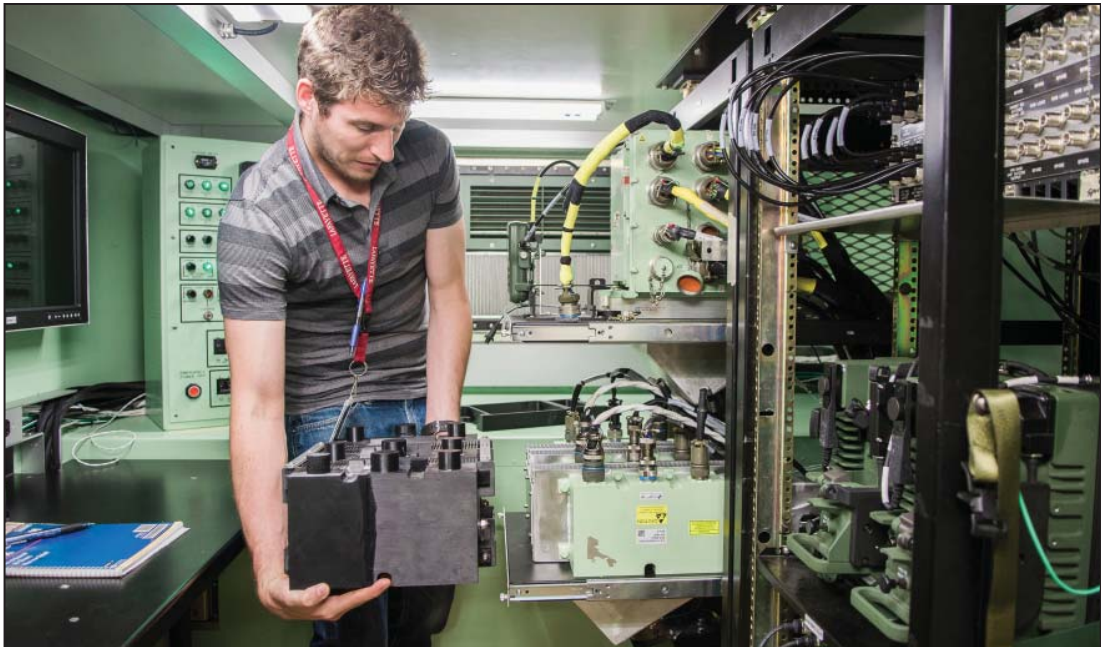
Mechanical Engineer Brian Thomas shows how a 3D-printed replica of a power supply looks exactly like the real thing. The model was used to help personnel make design modifications while waiting for the actual components to arrive on the depot. Thomas works in the Design Development and Fabrication Division.
