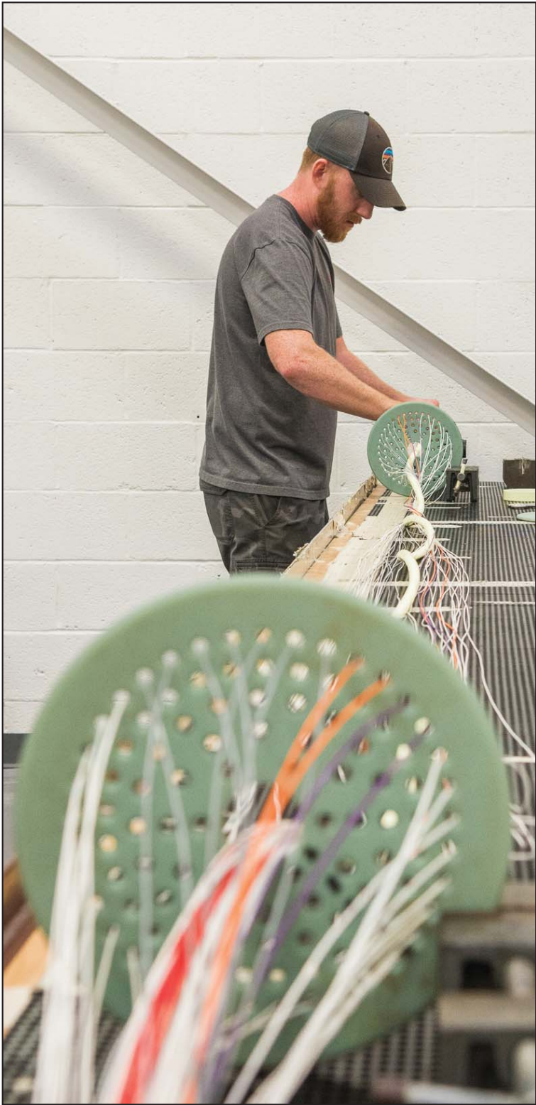
Electronics Worker Dave Horvath bundles a cable for the Common Remotely Operated Weapon Station (CROWS) diagnostic kit with the help of the perforated discs created using additive manufacturing. CROWS cables are unique and need to be fabricated by Tobyhanna. Horvath works in the Systems Integration and Support Directorate's Strategic Systems Cable Branch.
