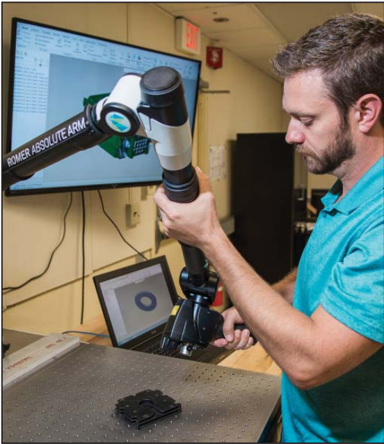
Left, Engineering Technician Mikael Mead uses a 3D scanner to capture data for reverse engineering purposes. The information is used to create drawings, 3D prints and manufacturing data. Above, Mead removes a model from the printer. Mead works in the Production Engineering Directorate's Design Development and Fabrication Division.
