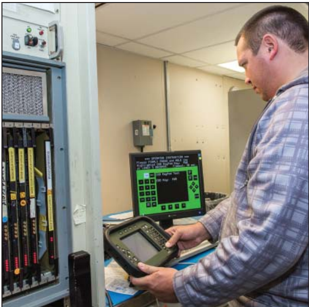
Justin Kubilus, electronics worker in the C4ISR Directorate’s TMDE Repair Section, does a final performance check on a chief of section display indicator (CSD).
