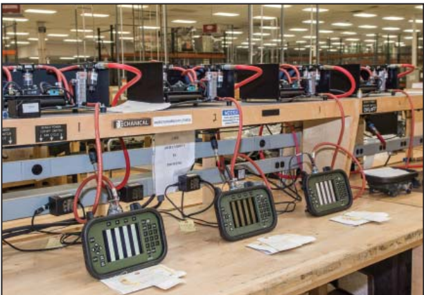
CSDs undergo a 48-hour purge to remove moisture from the displays prior to final assembly.
