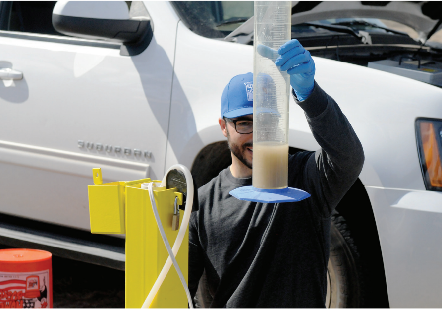
Matt Ellington | POST Pasquale Pozzolano, a contractor for the Environmental Protection Agency, collected water samples for testing from the permeable parking lot at Fort Riley’s Seitz Elementary School March 6. Basic safety tests are conducted on site and then samples are sent to a lab for additional testing for nitrate, metals, PH levels and oxygen absorption. The test determines if there are changes in water quality from permanent runoff testing sites at the permeable parking lot.
