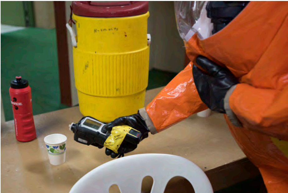
U.S. Army Sgt. Darwin Jurentkuff, survey team member, uses a MutliRAE Pro and RadEye to check for toxic chemicals and radiation.
