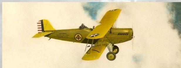
The most important aircraft in the 119th Observation Squadron’s early years was the Douglas O-2H. This rare colorized photo shows many features of this NJ National Guard aircraft, including the 0.3 caliber machine gun mounted in the rear cockpit, the perforated aluminum engine cowling and the “back-to-back 4s” insignia of the 44th Division. (NJDMVA photo)
