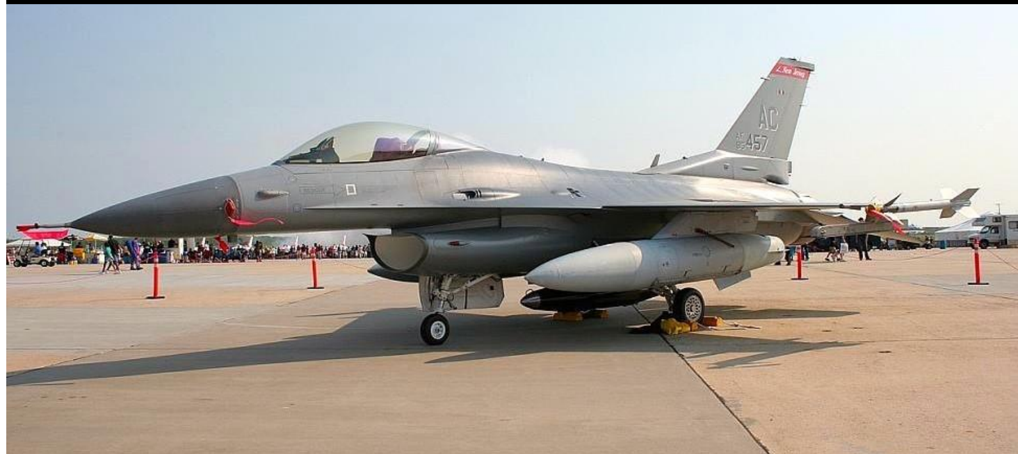
F-16C-Block 30A shown on the ramp at a McGuire AFB airshow is shown its GE/NSI inlet, hence its “Small-Mouth” denotation. (F16.net)
