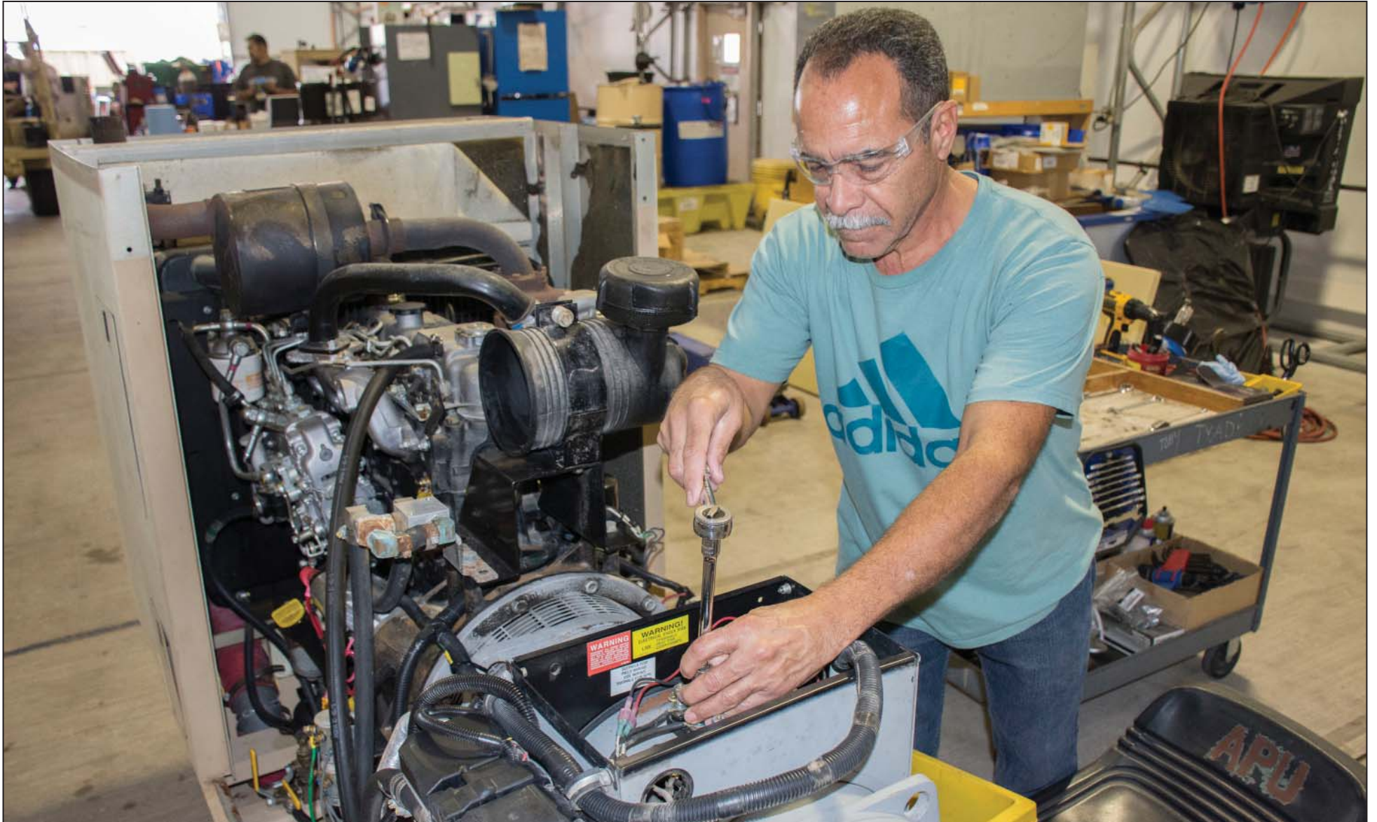
Roberto Duperon, air conditioner repairman in the C4ISR Directorate's Central Reset Section, makes repairs to the auxillary power unit on a medium Trailer Mounted Support System. (Photo by Justin Eimers)
