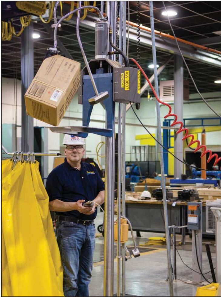
Left, Jeff Case, packaging specialist in the Logistics Support Activity Packaging, Storage and Containerization Center, conducts a drop test to determine if the package meets packaging performance requirements. Above, Electronics Engineer Clinton Holder aligns an optical stack used in testing the M2A2 Aiming Circle. Holder works in the Production Engineering Directorate's Avionics and Sensors Engineering Branch. (Photos by Jim Lentz)
