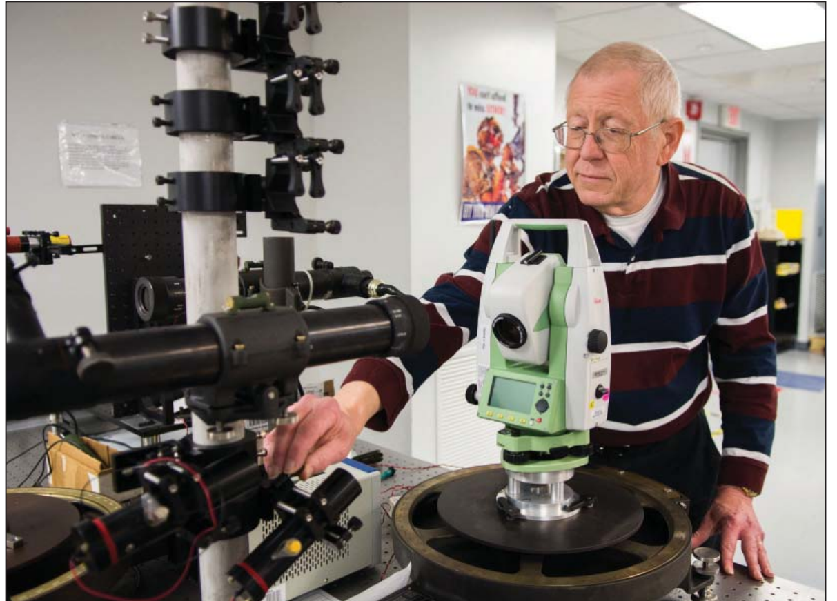
Left, Jeff Case, packaging specialist in the Logistics Support Activity Packaging, Storage and Containerization Center, conducts a drop test to determine if the package meets packaging performance requirements. Above, Electronics Engineer Clinton Holder aligns an optical stack used in testing the M2A2 Aiming Circle. Holder works in the Production Engineering Directorate's Avionics and Sensors Engineering Branch. (Photos by Jim Lentz)
