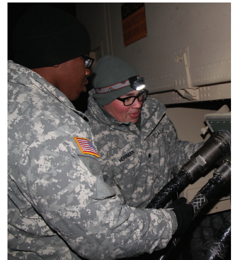
Specialist Tyler Hoffman right, patriot missile operator, and Spc. Deiontay Dawson, network systems operator-maintainer, both with Battery D, 1-43 ADA connect power cables to the AN/MPQ-65 radar set during the emplacement phase of their ballistic missile defense exercise, Feb. 8 on Osan Air Base, South Korea. (U.S. Army photo by Staff Sgt. Kelly S. Carlton, 35th ADA Public Affairs)
