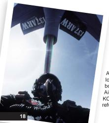
An F-16 pilot looks up at the fuel boom of a 137th Air Refueling Wing KC-135 during a refueling mission.
