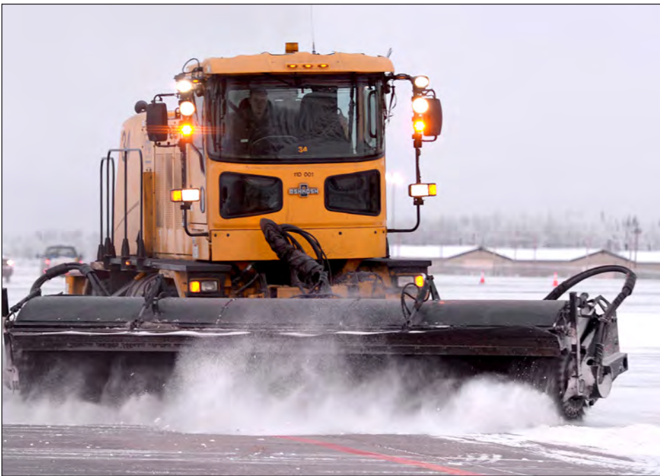
Airman 1st Class Seth Bryson, a 354th Civil Engineer Squadron pavement and construction equipment operator, steers a snow broom which removes snow from the flight line's taxiway Dec. 1, at Eielson Air Force Base, Alaska. During the snow season, these brooms operate 24 hours a day to keep the flight line clear for aircraft. (Photo by Airman Eric M. Fisher, 354th Fighter Wing Public Affairs)
