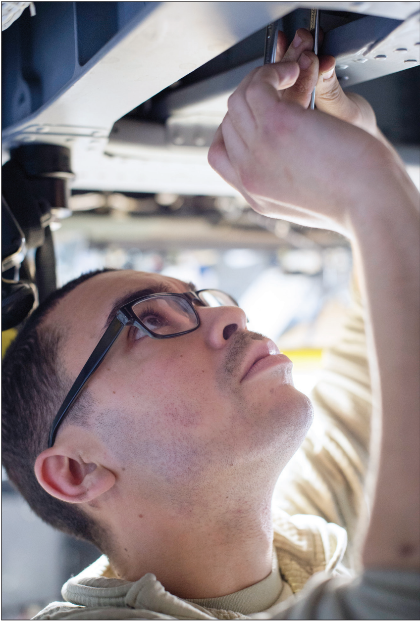
Alaska Air National Guard Airman 1st Class Mac Spurlock, an aerospace propulsion mechanic assigned to the 176th Maintenance Squadron, inspects an HC-130 Hercules engine at Joint Base Elmendorf-Richardson, Nov. 16. The HC-130s is undergoing an isochronal inspection to ensure the aircraft is safe and remains mission ready. (U.S. Air Force photos/Alejandro Pena)
