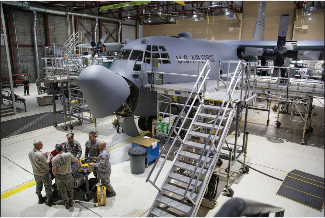
ABOVE: 176th MXS Airmen perform an isochronal inspection of a HC-130, Nov. 16. LEFT and RIGHT: Alaska Air National Guard Staff Sgt. Rafie Baez, a helicopter maintenance mechanic assigned to the 176th Maintenance Squadron, services a HH-60 Pave Hawk, Nov. 16. The Pave Hawk is undergoing a phase inspection to ensure the aircraft is safe and remains mission ready.
