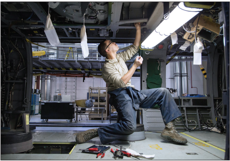
ABOVE: 176th MXS Airmen perform an isochronal inspection of a HC-130, Nov. 16. LEFT and RIGHT: Alaska Air National Guard Staff Sgt. Rafie Baez, a helicopter maintenance mechanic assigned to the 176th Maintenance Squadron, services a HH-60 Pave Hawk, Nov. 16. The Pave Hawk is undergoing a phase inspection to ensure the aircraft is safe and remains mission ready.
