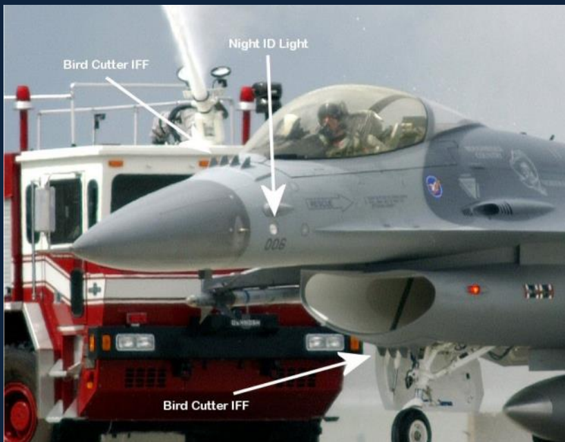
The F-16 ADF in this photo shows of its 150,000 candlepower spot light and unique 4-bladed "bird slicer" (also known as "bird cutter") advanced IFF antennae. (F16.net)
