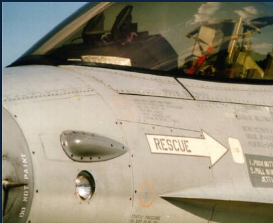
This close up photo of a F-16 ADF Vipers shows the 150,000 candle power spot-light in good details; it was used for night time visual identification of bogies. (F16.net)
