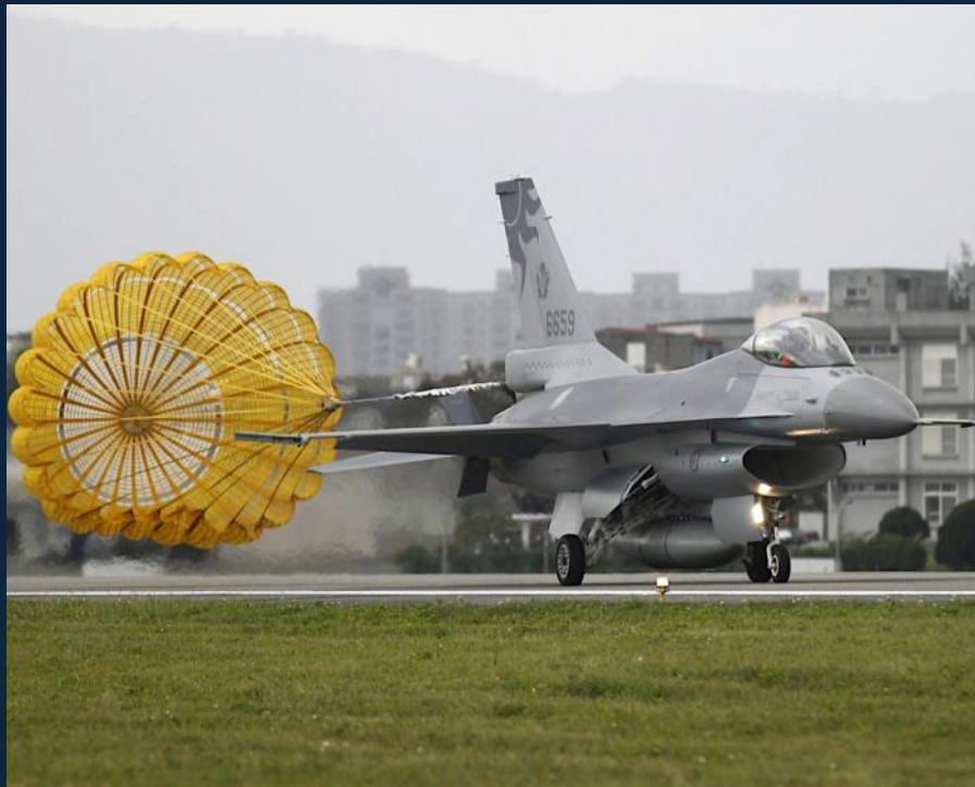
A Republic of China (Taiwanese) Air Force F-16A Block 20 Viper of the 401st Tactical Composite Wing uses its drag chute upon landing at Hualien AB. (F16.net)
