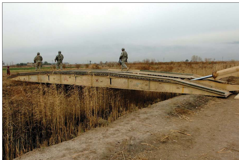
Combat engineers with Co. E, 1-30th Inf. Regt., 2nd BCT, 3rd Inf. Div., walk across the armored vehicle-launched bridge in Arab Jabour during Operation Acheron. The bridge makes a 35-foot gap passable for tactical vehicles.
