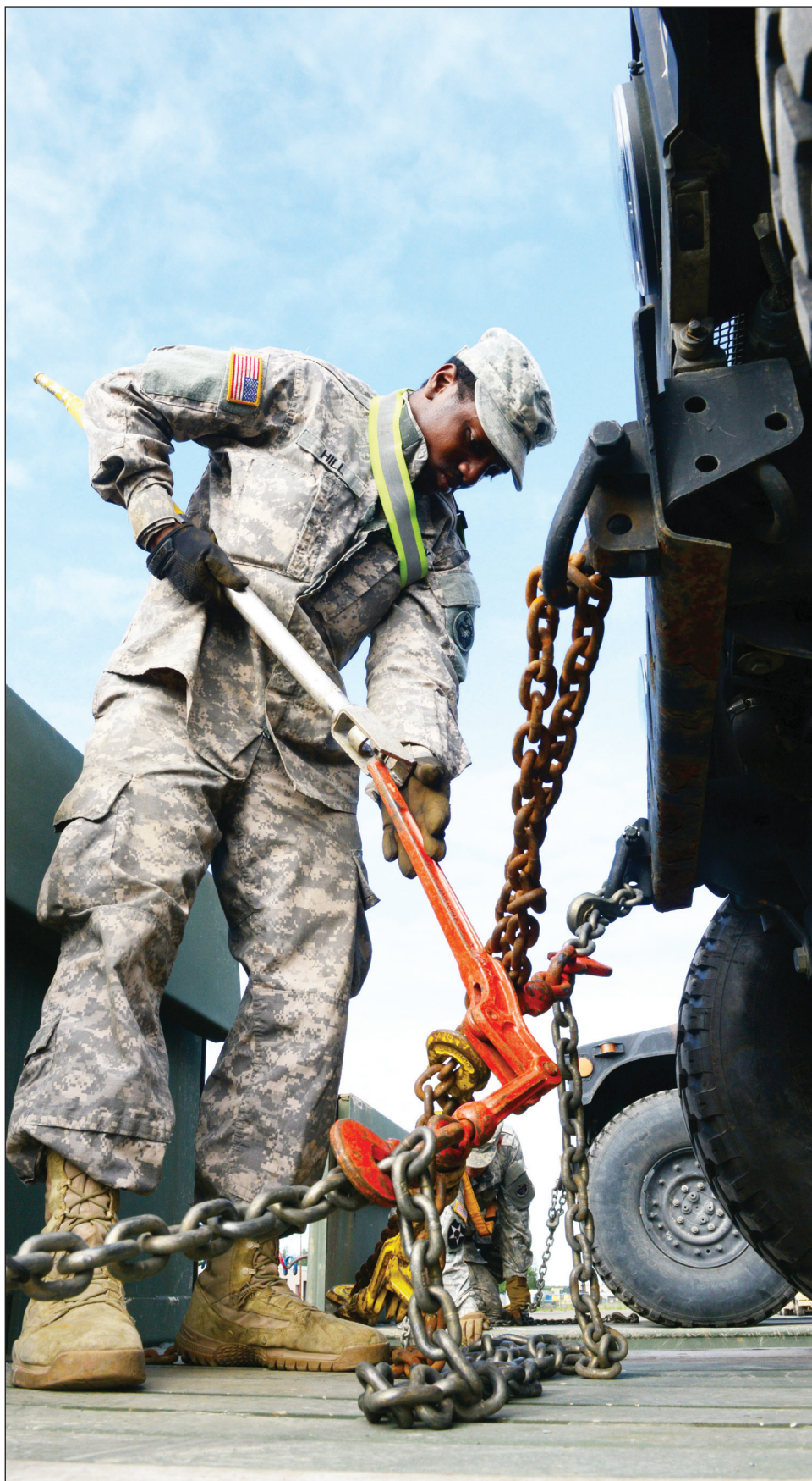
Pfc. Andrew Hartfield, a light transporter with the 539th Composite Truck Company from Fort Wainwright, uses a load binder to secure a Humvee (U.S. Air Force photos/Airman 1st Class Javier Alvarez)
