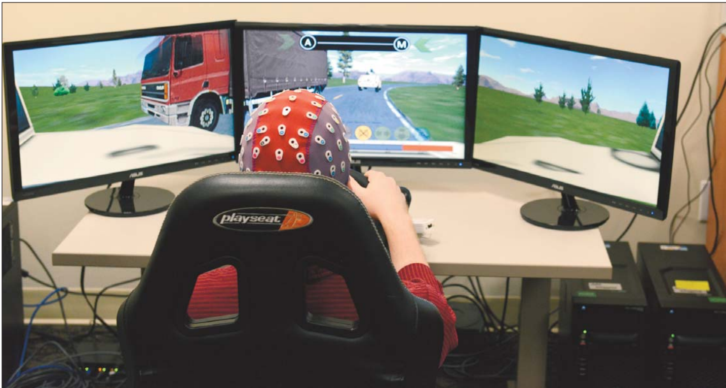
A car simulator at the U.S. Army Research Laboratory at Aberdeen Proving Ground, July 28, shows EEG sensors and caps used to monitor test subjects’ brain wave patterns while driving.
