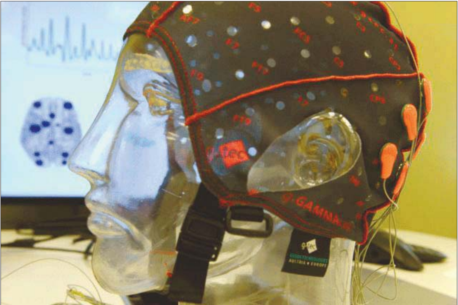
EEG sensors and cap used to monitor test subjects' brain wave patterns is shown mocked up, with brain wave patterns in the background. According to U.S. Army Research Laboratory scientists, advances in brain science could lead to improvements in performance and decision making, changing the way Soldiers fight in the near future.
