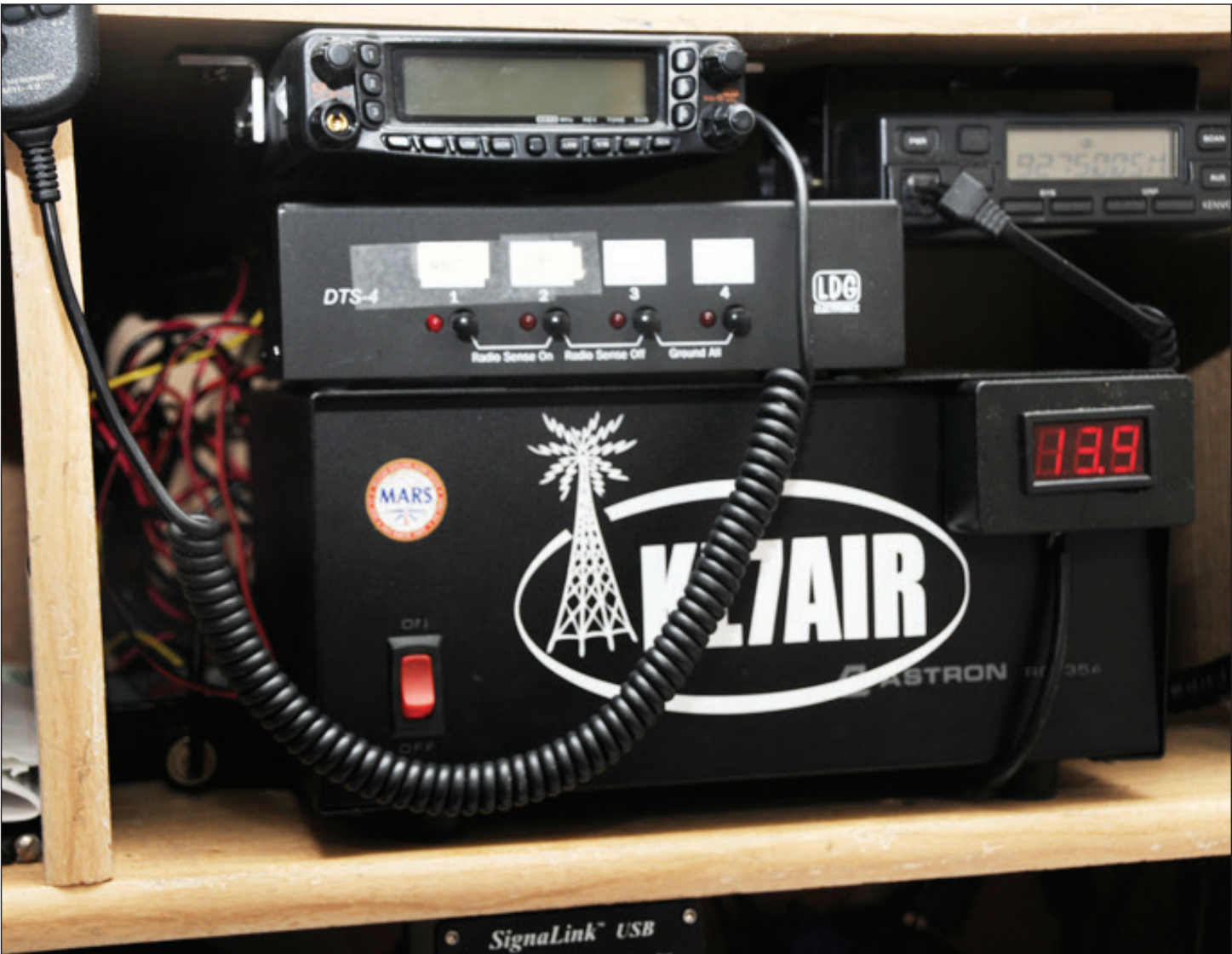
The power supply, antenna tuner, and a ham radio in the Elmendorf Amateur Radio Society ham shack in the Civil Air Patrol building. Ham radio is a relatively inexpensive hobby and can be used both for fun and for relaying information or contacting help in an emergency. (U.S. Air Force photo/Chris McCann)
