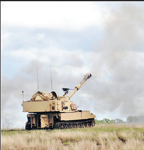
Staff Sgt. Warren W. Wright Jr. | 1ST ABCT LEFT: An M109A6 Paladin from 1st Battalion, 5th Field Artillery Regiment, 1st Armored Brigade Combat Team, 1st Infantry Division, fires a conventional 155mm round equipped with the XM1156 precision guidance kit during familiarization training April 30 at a Fort Riley training area. The PGK system allows for increased accuracy of conventional rounds, greatly reducing the possibility of collateral damage. RIGHT: A pair of M2 Bradley Fighting Vehicles from Company C, 1st Battalion, 16th Infantry Regiment, 1st Armored Brigade Combat Team, 1st Infantry Division, participate in a live-fire exercise May 6 at a Fort Riley Training Area as an AH-64 Apache from the 1st Combat Aviation Brigade, 1st Inf. Div., flies overhead. The event was a part of operation Danger Focus, a month-long exercise designed to prepare the “Devil” brigade for its upcoming rotation to the National Training Center at Fort Irwin, California.
