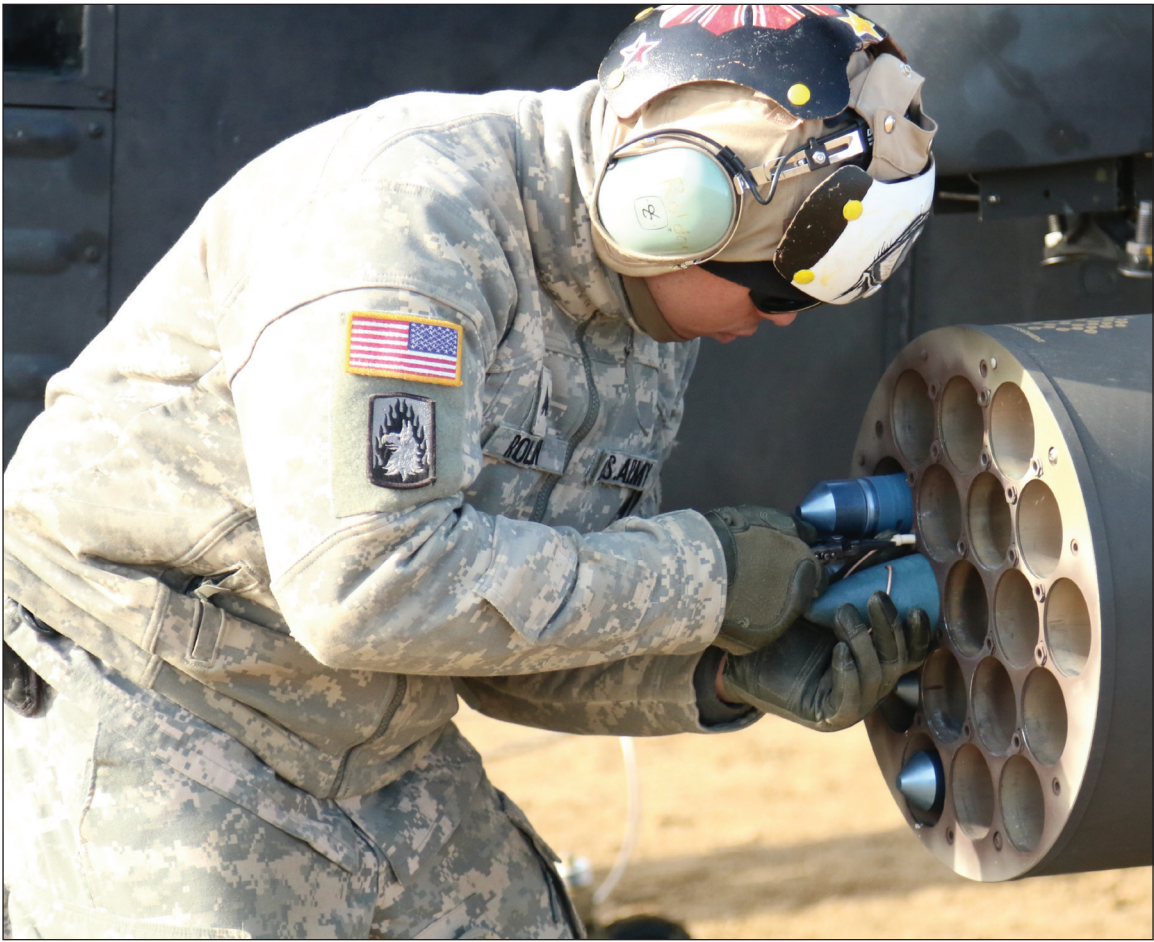
Sgt. Franzwillie Roldan, an AH-64D Armament/Electrical/Avionics Systems Repairer in 1st Attack Reconnaissance Battalion, 25th Combat Aviation Brigade places a training missile into an Apache wing rocket missile pod April 4, 2016 at the Forward Area Rearming Point at Yukon Training Area. (U.S. Army photo/Spc. Samantha L. Magers)
