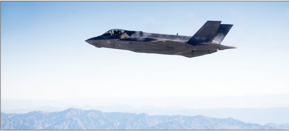
An F-35 Lightning II test pilot fires the four-barrel 25 mm GAU-22/A Gatling gun while in flight Oct. 30 over China Lake Weapon Range, Calif. (U.S. Air Force photo/Chad Bellay)
