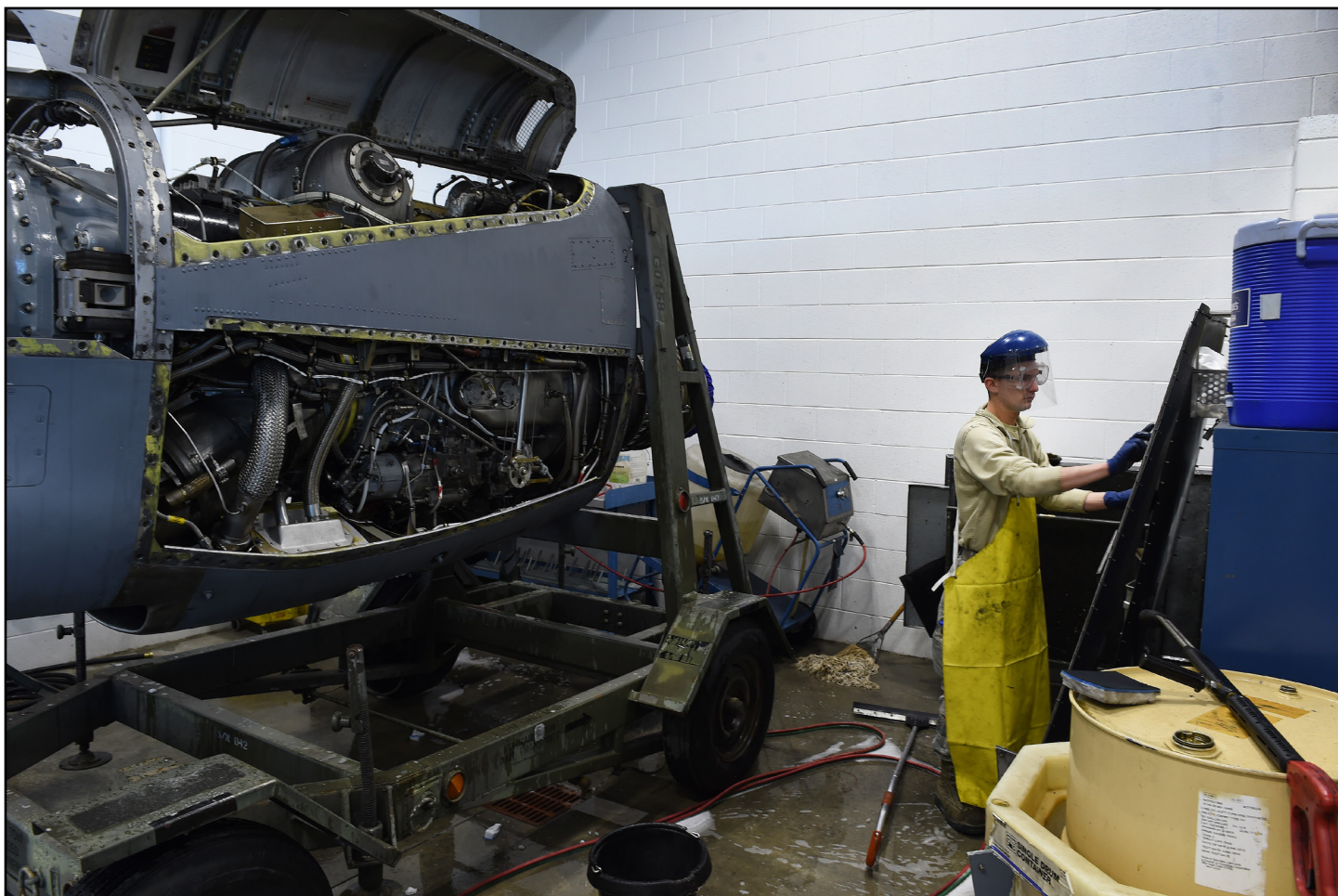
Staff Sgt. Wayne Wheeler, an aerospace propulsion technician with the 153rd in Cheyenne, washes a C-130 engine panel.
