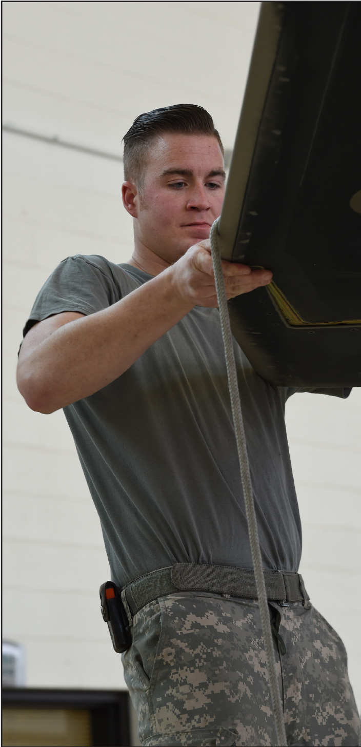
Army Sgt. Phil Buettner, a crew chief at C Company, 5th Battalion, 159th Aviation Regiment, replaces a main rotor blade tip on a UH-60 Black Hawk at the Army Aviation Support Facility, in Cheyenne.
