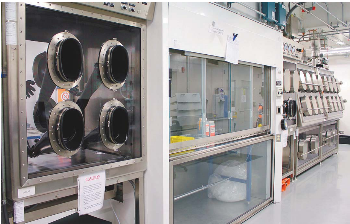
The Non-Traditional Agent Defense Test System. The system is a collection of specialized test chambers designed to test chemical agent protection, detection and decontamination equipment under operational conditions most relevant to today’s warfighter.
