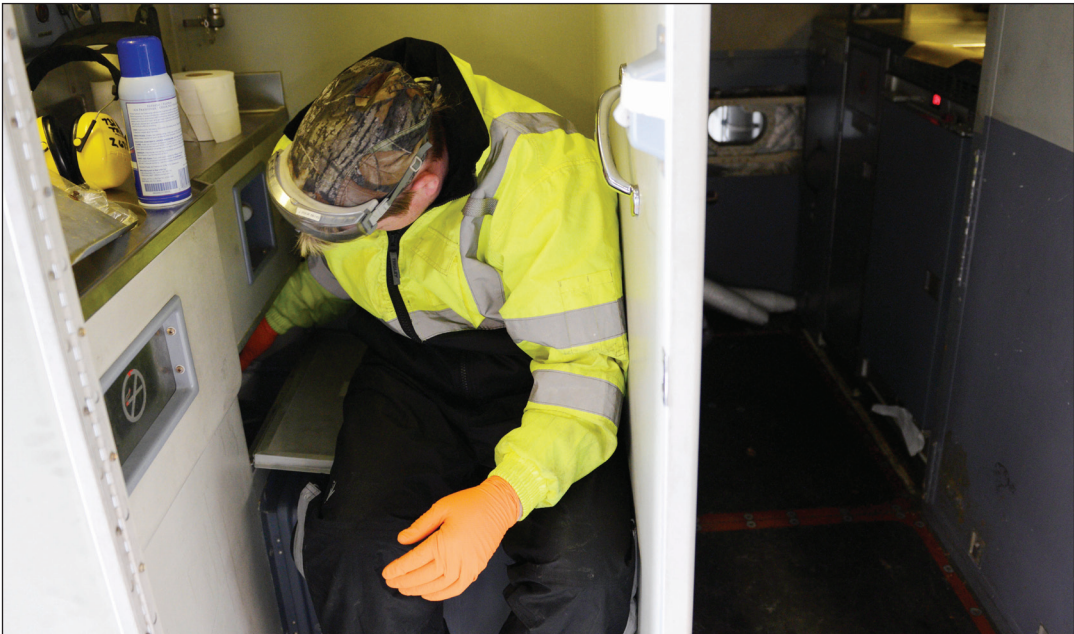
ABOVE: Jeffrey Zook, left, and Lewis Come attach a drainage tube to a C-17 Globemaster III at Joint Base Elmendorf-Richardson, to remove waste from the aircraft’s lavatory. The 732nd Air Mobility Squadron’s Fleet services Airmen not only clean and empty lavatories, they remove trash and prepare outbound aircraft with pillows, blankets and other items. Zook is a fleet services vehicle operator and Come is the fleet services supervisor. (U.S. Air Force photos/Airman Valerie Monroy) LEFT: Jeffrey Zook, 732nd Air Mobility Squadron fleet services vehicle operator, assists with the draining of the lavatory on a C-17 Globemaster III. The service provided by fleet services varies by aircraft.
