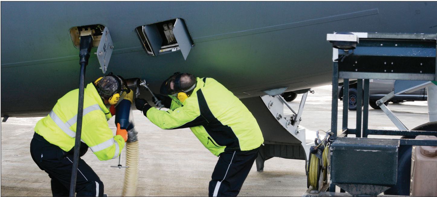
ABOVE: Jeffrey Zook, left, and Lewis Come attach a drainage tube to a C-17 Globemaster III at Joint Base Elmendorf-Richardson, to remove waste from the aircraft’s lavatory. The 732nd Air Mobility Squadron’s Fleet services Airmen not only clean and empty lavatories, they remove trash and prepare outbound aircraft with pillows, blankets and other items. Zook is a fleet services vehicle operator and Come is the fleet services supervisor. (U.S. Air Force photos/Airman Valerie Monroy) LEFT: Jeffrey Zook, 732nd Air Mobility Squadron fleet services vehicle operator, assists with the draining of the lavatory on a C-17 Globemaster III. The service provided by fleet services varies by aircraft.
