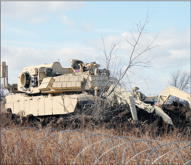
“Diehard” Soldiers with the 1st Engineer Battalion, 1st Armored Brigade Combat Team, 1st Infantry Division, man the Assault Breacher Vehicle and sweep for landmines during a training exercise Feb. 3 at Fort Riley. This ABV utilizes a full width mine plow in order to remove mines from the ground. The blades have three positions for depth.
