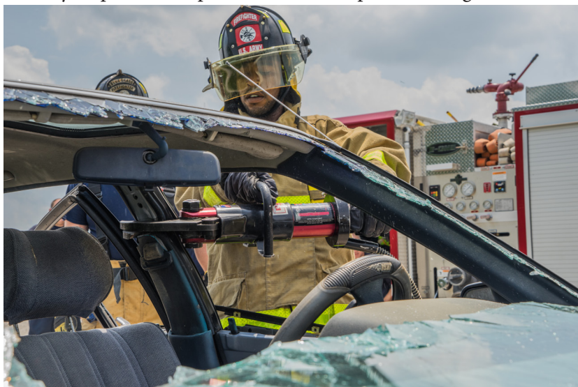
Spc. Mark Brooks cuts into the door jamb of a junk car with the Jaws of Life to practice safe and controlled techniques to rescue car accident victims at Blue Grass Army Depot, Ky., June 9th.
