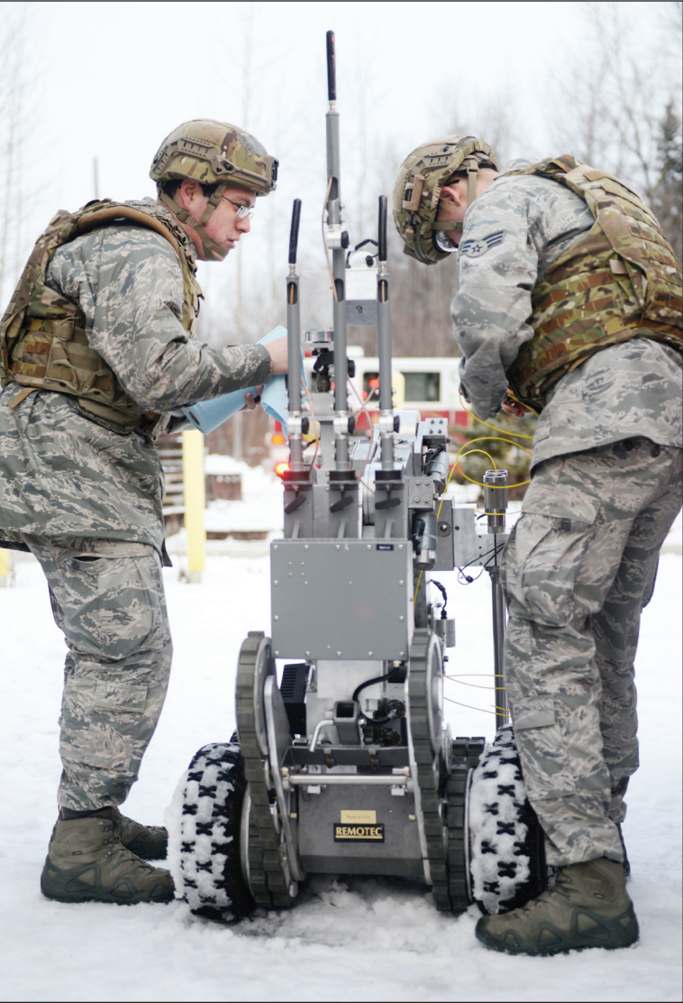
Airmen prepare an F6 robotic platform as part of a training exercise on Joint Base Elmendorf-Richardson Jan. 27. The F6 has a wide range of capabilities for many types of explosive ordnance disposal missions. (U.S. Air Force photo/Airman 1st Class Javier Alvarez)
