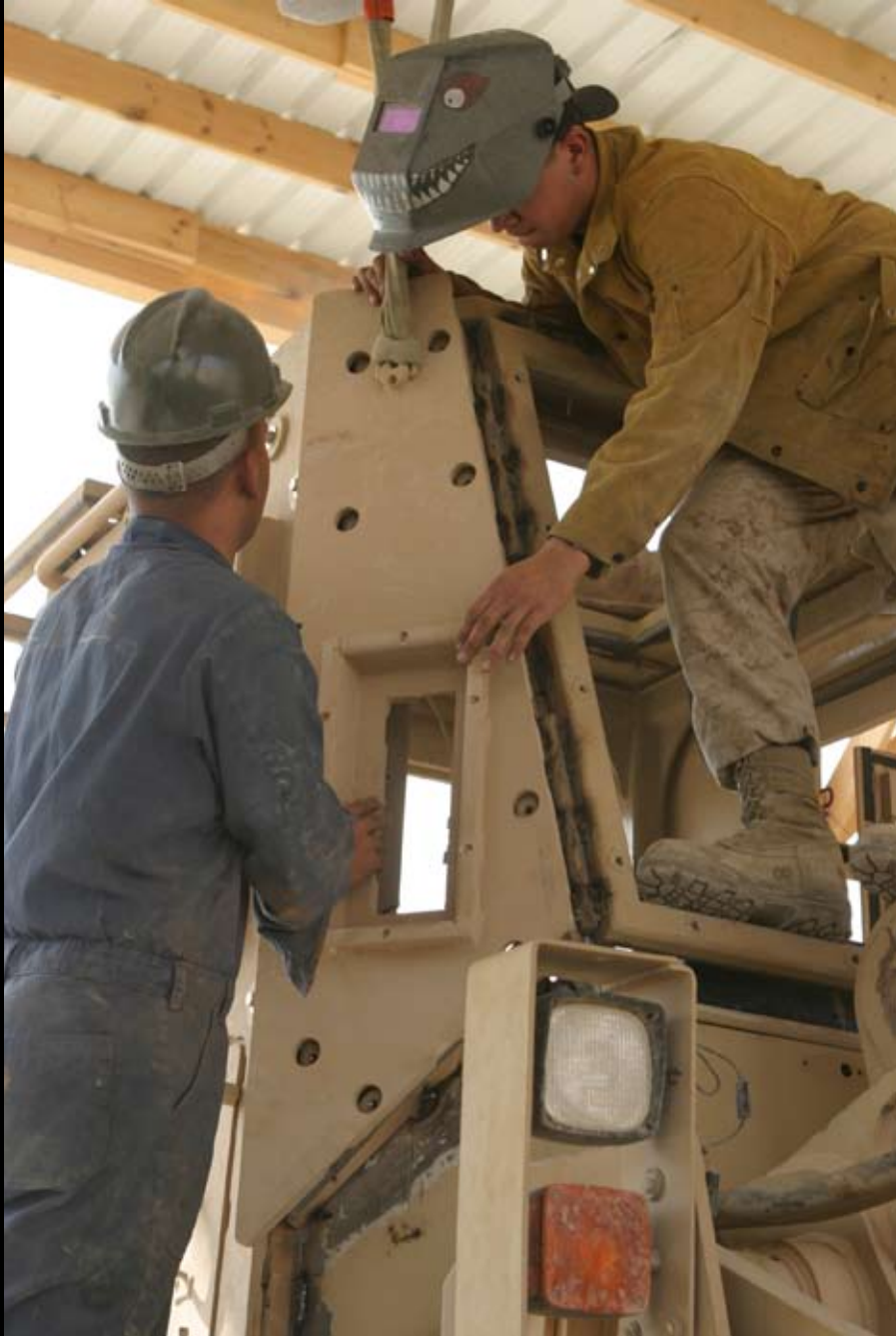
Top left: Marine Lance Cpls. Ivan Gonzalez and Randy Ames prepare to weld the frame of an armor kit to a TRAM at Al Asad Air Base Oct. 10. Photo by Marine Lance Cpl. Abby Burtner.
