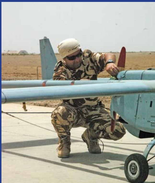
An electronic technician with Romanian Army Military Intelligence performs preflight checks on a Shadow 600 unmanned aerial vehicle prior to launching it.
