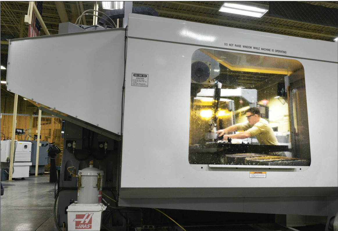
ABOVE: Air Force Staff Sgt. Jeremy Hamblin, 3rd Maintenance Squadron, Aircraft Metals Technology Flight craftsman, measures inconsistencies on a plastic mold in the Aircraft Metals Technology building November 24. After measuring the discrepancies, Hamblin can plug the data into the system to ensure they are not replicated on the aluminum billet. (U.S. Air Force photos/Airman 1st Class Kyle Johnson) LEFT: Hamblin machines a part in a closed environment.
