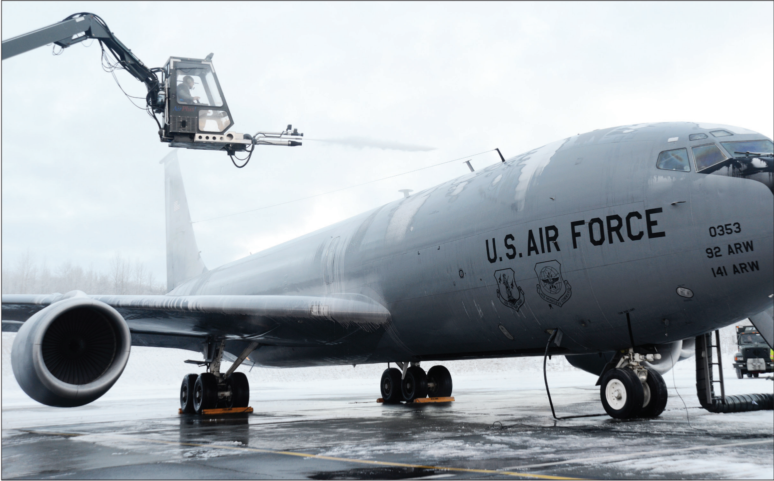
Air Force Staff Sgt. Tyler Derr, 732nd Air Mobility Squadron avionics specialist, deices a KC-135 Stratotanker from Fairchild Air Force Base on the flight line at Joint Base Elmendorf-Richardson Dec. 3. There is always a person in the truck, one in the deicer and one on the ground to make sure the aircraft is deiced all around. (U.S. Air Force photo/Airman 1st Class Christopher R. Morales)
