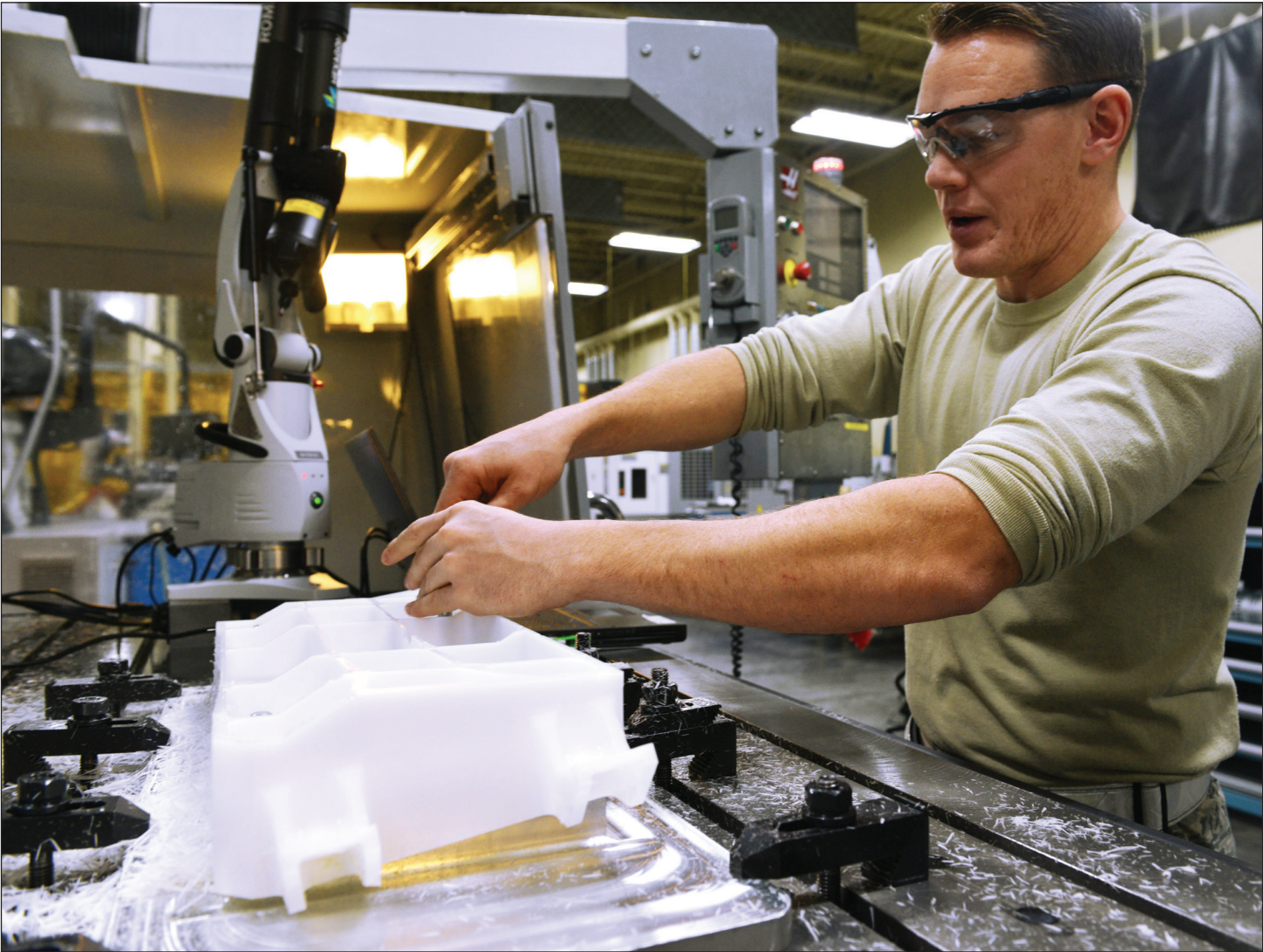
ABOVE: Air Force Staff Sgt. Jeremy Hamblin, 3rd Maintenance Squadron, Aircraft Metals Technology Flight craftsman, measures inconsistencies on a plastic mold in the Aircraft Metals Technology building November 24. After measuring the discrepancies, Hamblin can plug the data into the system to ensure they are not replicated on the aluminum billet. (U.S. Air Force photos/Airman 1st Class Kyle Johnson) LEFT: Hamblin machines a part in a closed environment.
