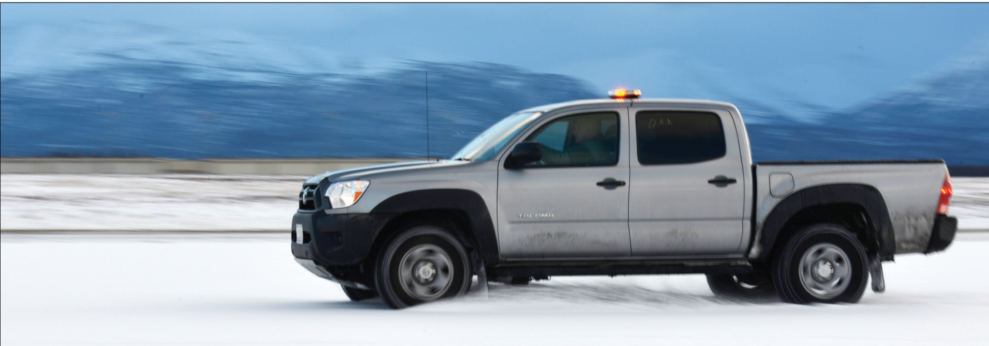
TOP: Senior Airman Jerred Johnson, Airfield Management operations supervisor with the 3rd Operations Support Squadron, checks his decelerometer after inducing a skid on the Joint Base Elmendorf-Richardson flightline Nov. 9. By reading how the vehicle performs in the brake, the decelerometer quantifies the friction level of the runway in a measurable way.
