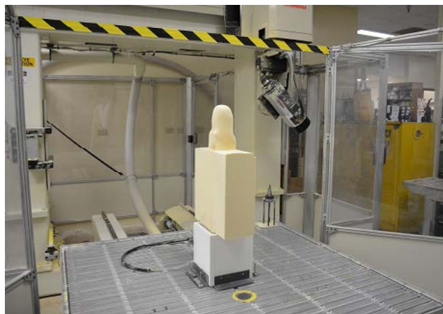
Once a 3-D computer model of a prosthetic is made, it is carved using the computer aided carver. (Photo by Emily Yeh)
