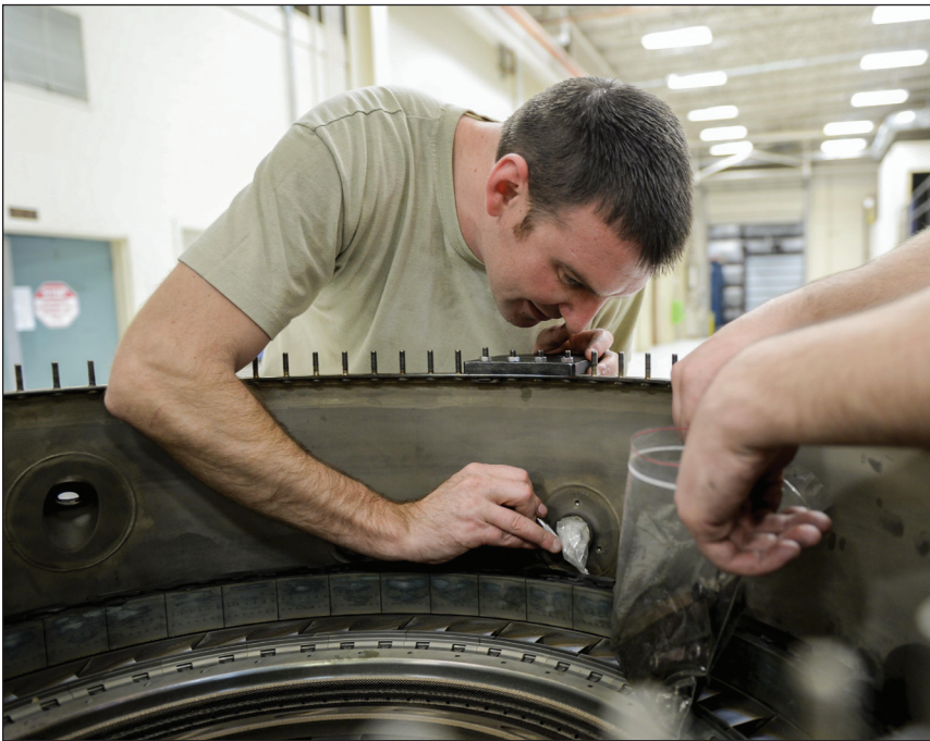
ABOVE: Air Force Staff Sgt. Jonathan Royder, a 354th Maintenance Squadron aerospace propulsion craftsman, extracts bolts from a combustion diffuser nozzle assembly Oct. 8 at Eielson Air Force Base. (U.S. Air Force photos/Senior Airman Peter Reft) LEFT: Senior Airman Cody Bowman, a 354th MXS aerospace propulsion journeyman, services a jet engine compressor during an engine rebuild in the Engine Shop at Eielson Air Force Base. Bowman disassembled the compressor for a fan blade inspection.
