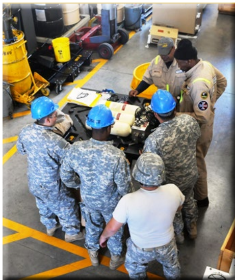
Field Level Maintenance New Equipment Training instructors (top) teach Soldiers from the 355th Chemical Company, how to disassemble nitrogen tanks from the Height Management System of a Nuclear, Biological, Chemical, Reconnaissance Vehicle Stryker, during FLMNET instruction, May 8, at Joint Base Lewis-McChord, Wash.
