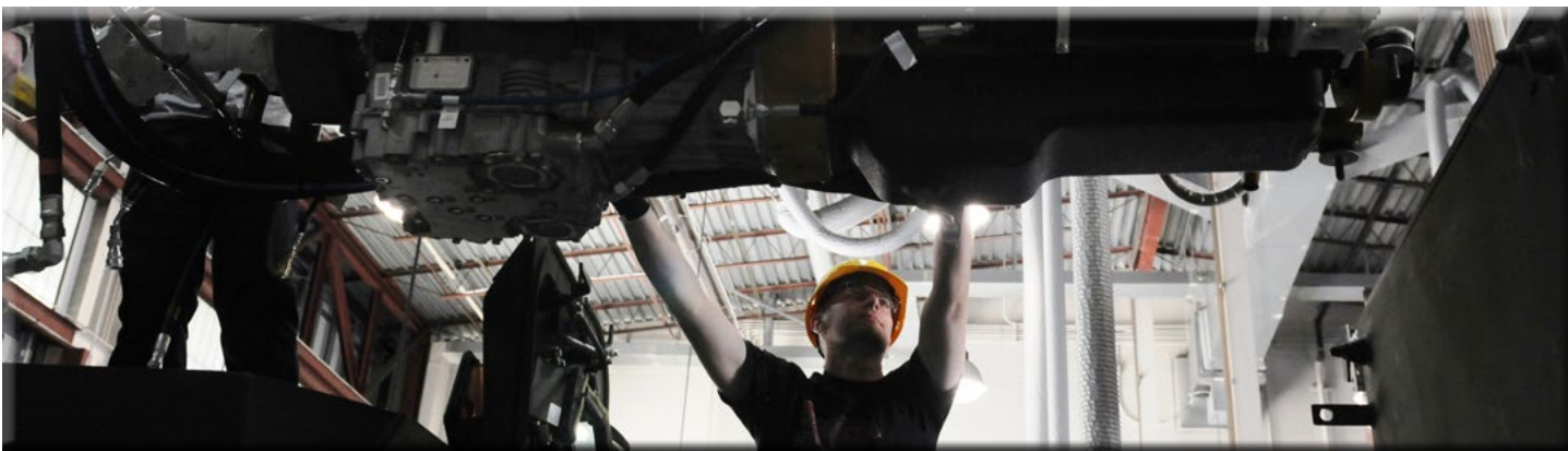
A mechanic for the 88th Regional Support Command guides the power pack belonging to a Nuclear, Biological, Chemical, Reconnaissance Vehicle (NBCRV) Stryker into place, during Field Level Maintenance New Equipment Training (FLMNET) instruction, May 8, at Joint Base Lewis-McChord, Wash.
