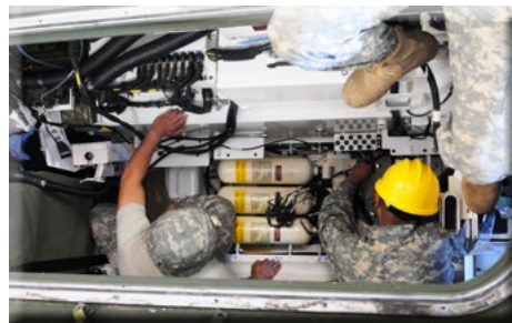
Soldiers from the 355th Chemical Company, based in Las Vegas, disassemble the Height Management System of a Nuclear, Biological, Chemical, Reconnaissance Vehicle Stryker, during Field Level Maintenance New Equipment Training, May 8, at Joint Base Lewis-McChord, Wash.
