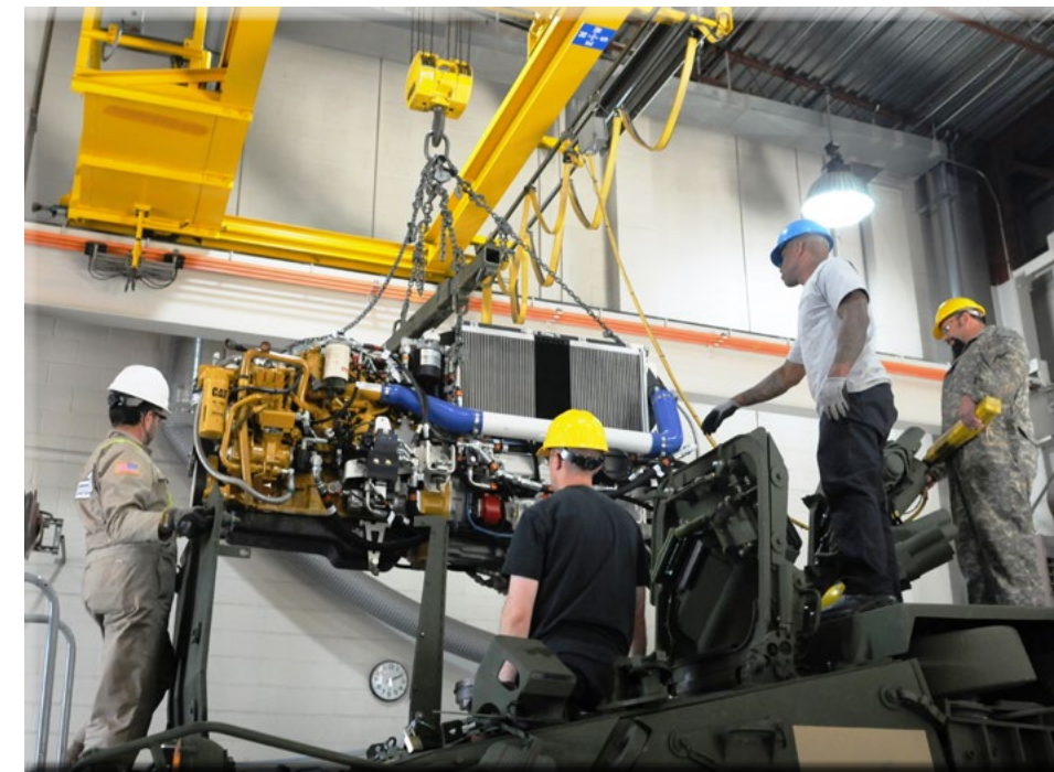
Melvyn Rosado (left), a Field Level Maintenance New Equipment Training instructor for General Dynamics, supervises the power pack belonging to a Nuclear, Biological, Chemical, Reconnaissance Vehicle Stryker being placed in the vehicle, while being observed by mechanics from the 88th Regional Support Command taking the course, during FLMNET instruction, May 8, at Joint Base Lewis-McChord, Wash.
