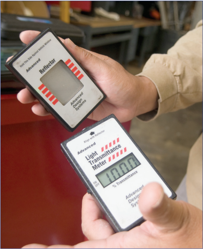
An automotive instructor at the Auto Skills Center shows the light meters used when inspecting vehicles with tinted windows at their temporary offices in building 1698, Monday. All vehicle tinting must meet guidelines set in Federal Motor Vehicle Safety Standards 205 and Chapter 291, Section 21.5 of the Hawaii Revised Statutes.
