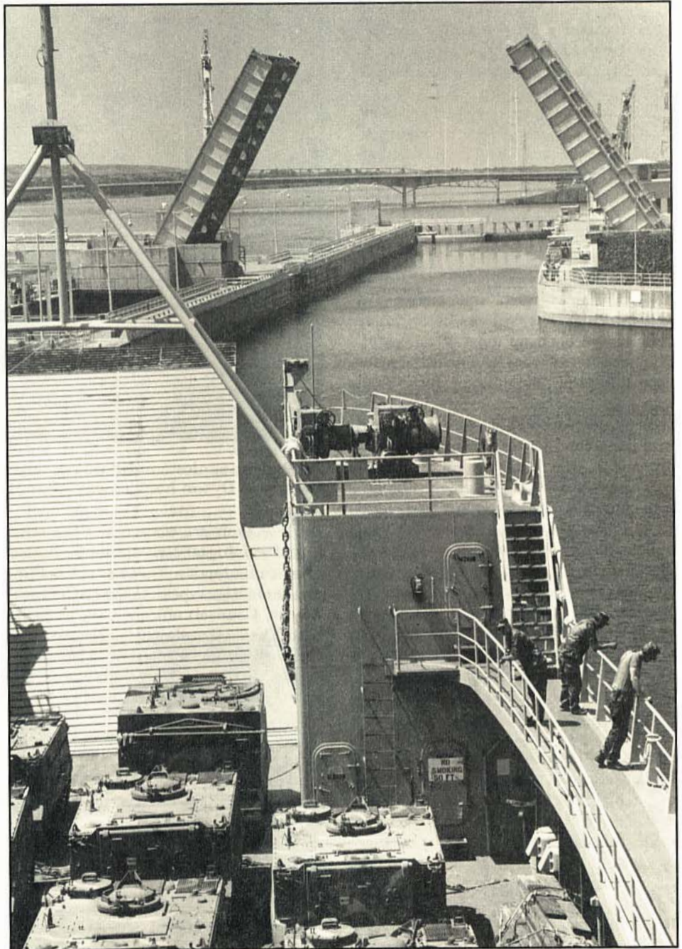
The Columbia's following current forced Somervell to drift sideways at the McNary Dam lock; bow thrusters straightened her out in time.
