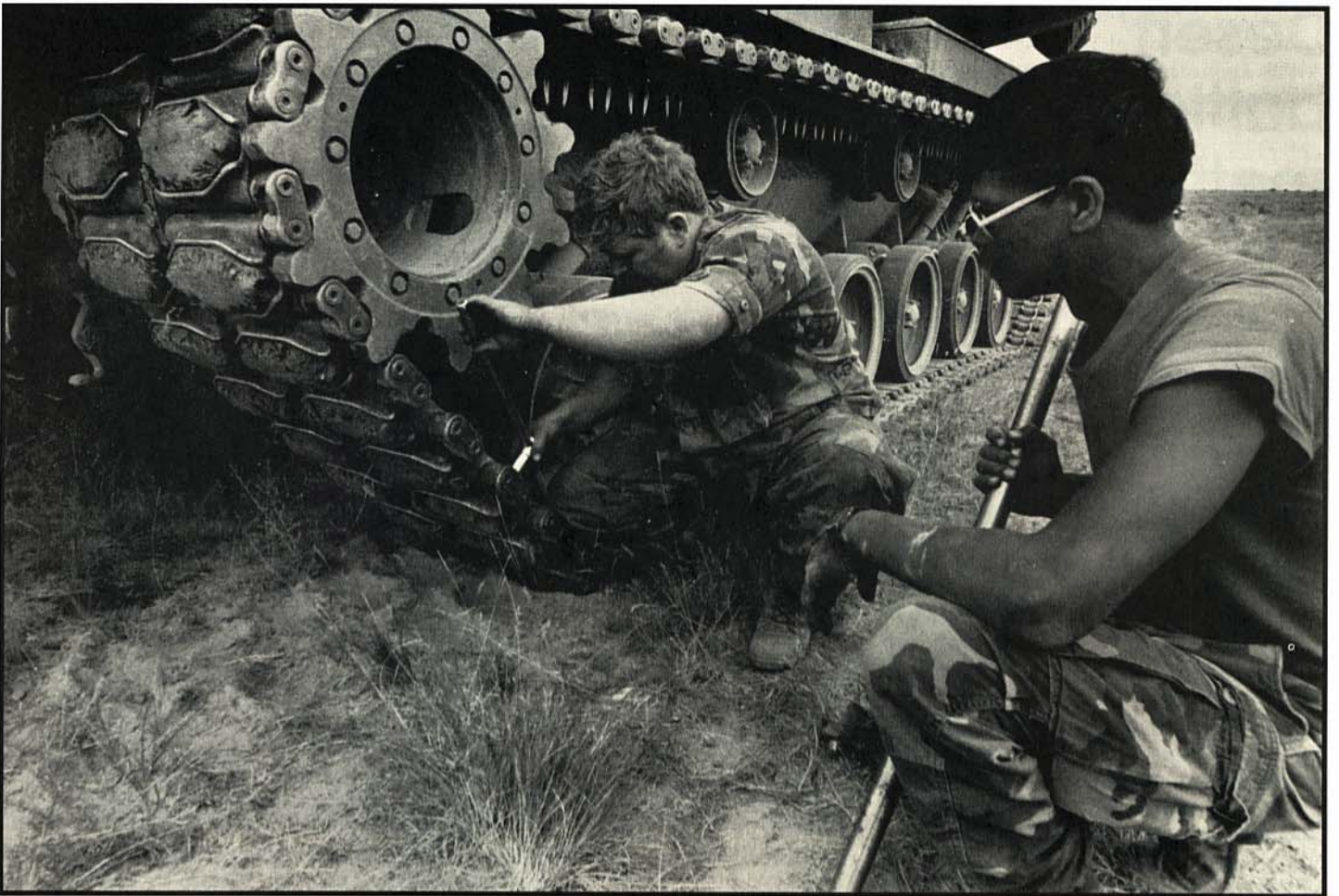
Sgt. Bob Valentine wrestles an end connector nut while Spec. William Ocho stands by to pry parts loose with a tank bar.
