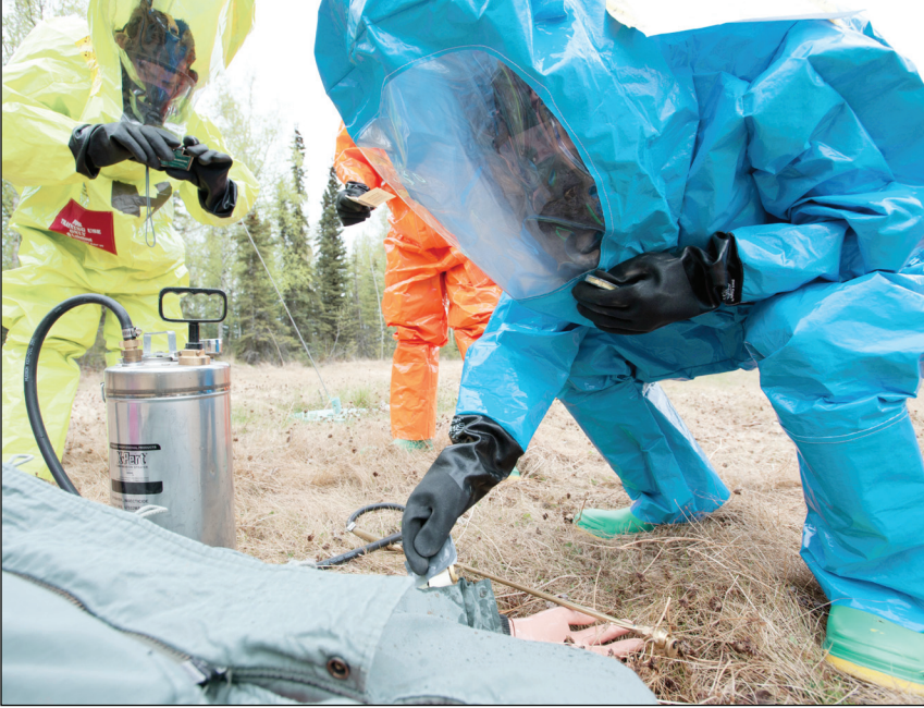
LEFT: Castellanos (foreground) dips M-8 and M-9 paper into chemicals on a simulated body to determine which contaminants are present as Senior Airman Alex Liccione examines used paper. Liccione is a 673d Aerospace Medicine Squadron bioenvironmental engineering technician and a native of New York, N.Y. RIGHT: Castellanos gets his first breath of fresh air after simulated decontamination. (U.S. Air Force photos/Tech. Sgt. Robert Barnett)
