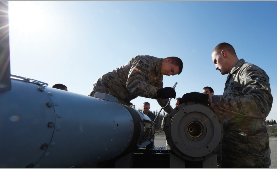
Senior Airmen Michael Crow (left) and Evan Kirchner, both assigned to the 3rd Munitions Squadron, attach strakes to a GBU-32 Joint Direct Attack Munition during combat munitions training at Joint Base Elmendorf-Richardson April 23. (U.S. Air Force photo/Staff Sgt. Sheila deVera)
