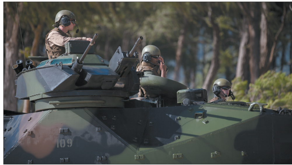
Marines sit atop the vehicle — driver, crew chief/vehicle commander, and turret gunner. Armament for the gunner includes a MK19 grenade launcher and the M2 .50-caliber heavy machine gun.
