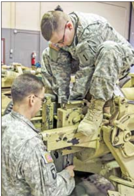
Spc. Anthony Garrett (left), and Pfc. Raymond Valdez, both assigned to Battery A, 2nd Bn., 32nd FA, 4th IBCT, 1st Inf. Div., exercise the recoil system of a M119A2 howitzer weapon system as part of the inspection criteria for Picatinny Arsenal at the battalion's motor pool Feb. 24 at Fort Riley.
