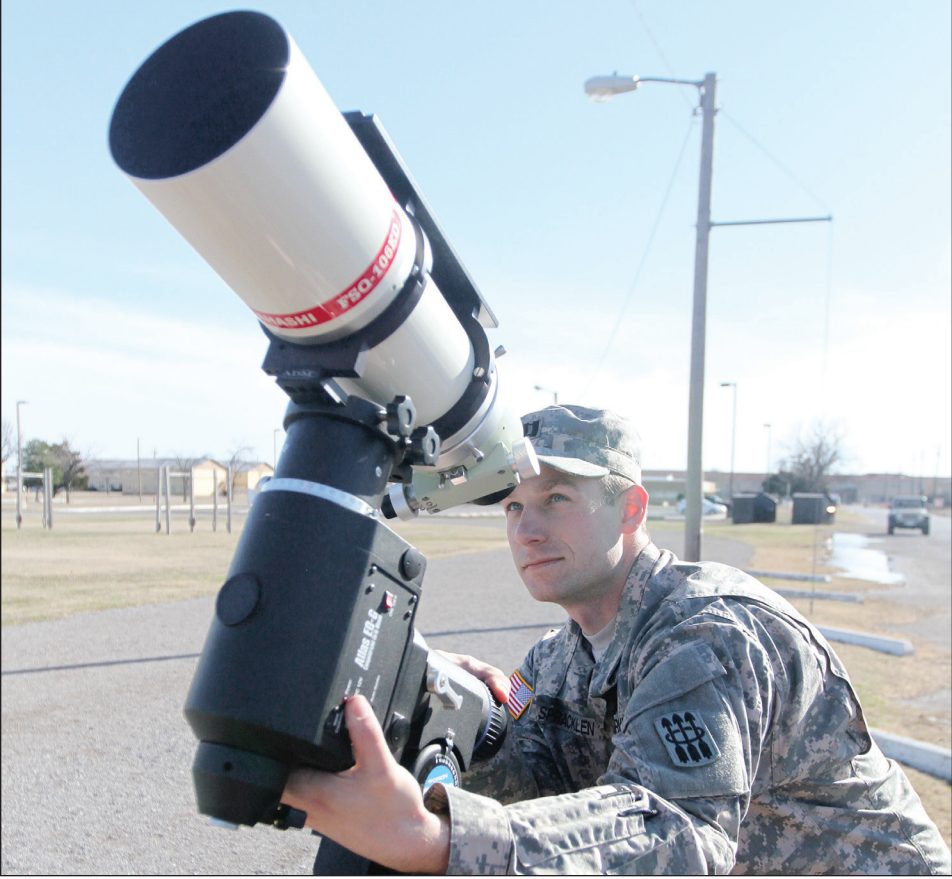
ABOVE: Army Capt. Joe Spracklen, an Air Defense Artillery Captains’ Career Course student at Fort Sill, Okla., uses a telescope, camera, guide scope, mount, tripod and a laptop for astrophotography. He also created a shield to diminish any disturbance in the photos from wind gusts. (U.S. Army photo/Marie Berberea)
